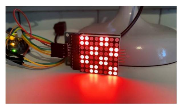
This intro to Arduino uses a LED matrix to show how to connect and use existing libraries to create fun projects without too much coding and wiring.
