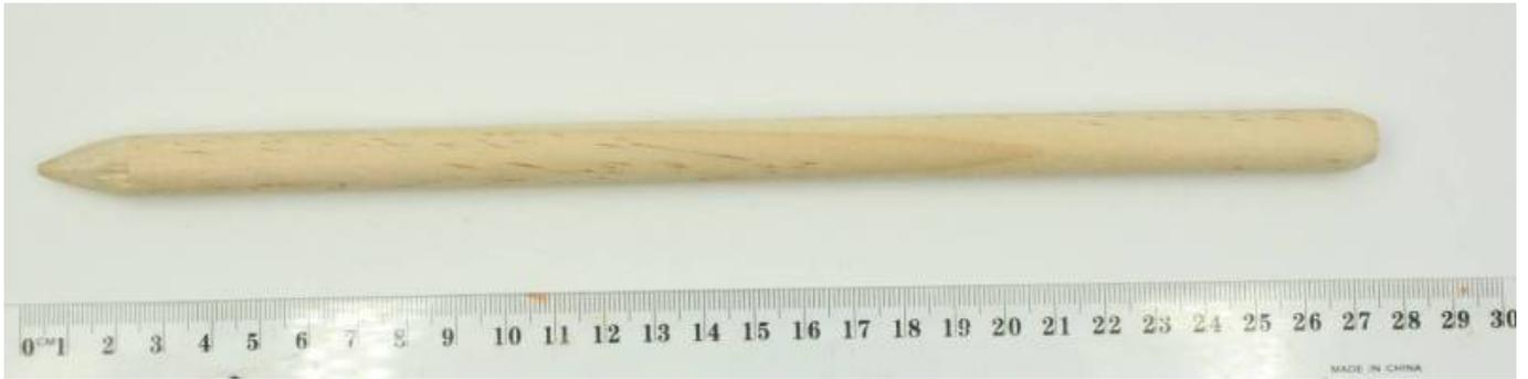
The drill stick needs to be at least 15mm diameter to be effective. Thinner material will smoke, but will not produce enough sawdust for ignition to occur. Because friction is desired, using dowel with a smooth circumference is better (grooved dowel may not work). Natural woods can be substituted, but straight pieces are required so that the drilling is easily controlled (and remove the bark).
