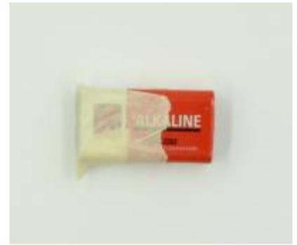
The 9V battery will work consistently, though a 1.5V battery (like a AA) will not have enough energy to work. If two 1.5V batteries are joined in series (+ to -) and held together with some tape, there may be enough power to set the steel wool alight.
