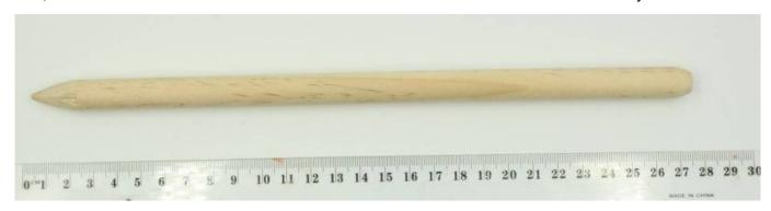
The drill stick needs to be at least 15mm diameter to be effective. Thinner material will smoke, but will not produce enough sawdust for ignition to occur. Because friction is desired, using dowel with a smooth circumference is better (grooved dowel may not work). Natural woods can be substituted, but straight pieces are required so that the drilling is easily controlled (and remove the bark).
