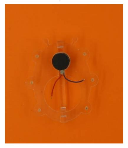
Remove the protective paper (white) from the vobromotor, and insert it into the small hole in the body. It should adhere to the backbone
