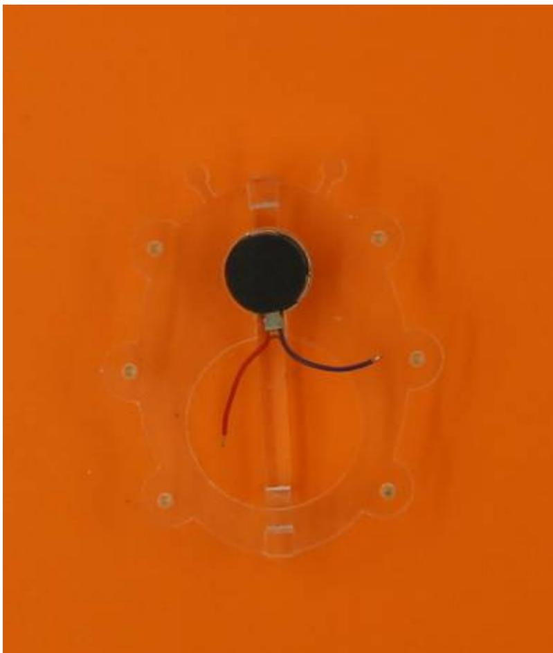
Remove the protective paper (white) from the vibromotor, and insert it into the small hole in the body. It should adhere to the backbone
