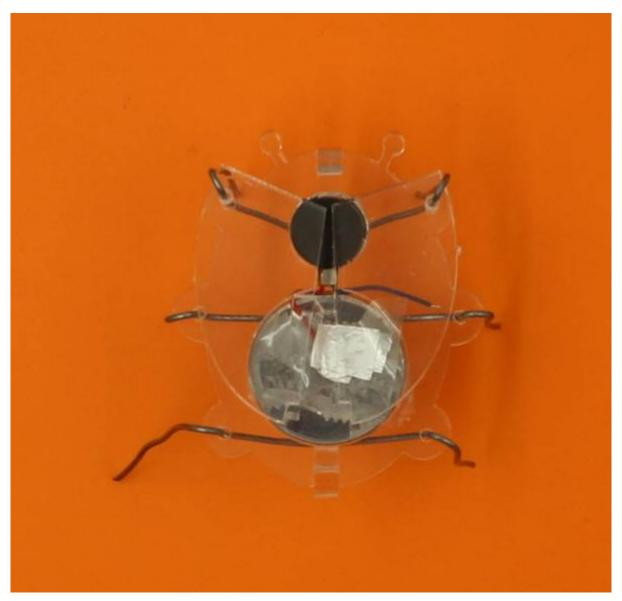
Wrap a piece of alfoil around the exposed end of the red wire, and use the sticky tape to attach it to the positive side of the battery (which should be on top). You vibrobot will now jiggle across a hard surface (until the battery goes flat).
