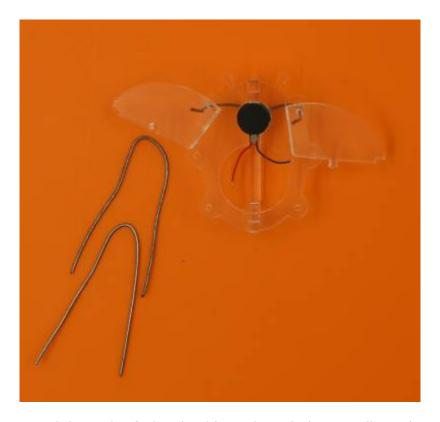
Turn the Vibrobot over and the ends of wire should now be pointing up. Slip a wing over each leg, using the small hole provided.
