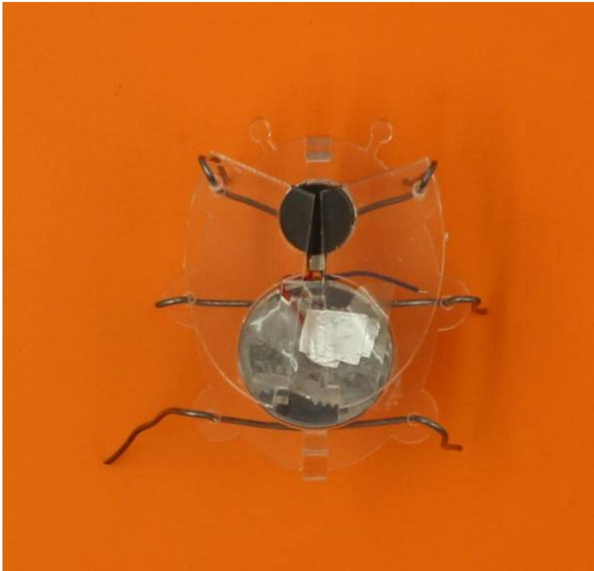
Wrap a piece of alfoil around the exposed end of the red wire, and use the sticky tape to attach it to the positive side of the battery (which should be on top). Your vibrobot will now jiggle across a hard surface (until the battery goes flat).
