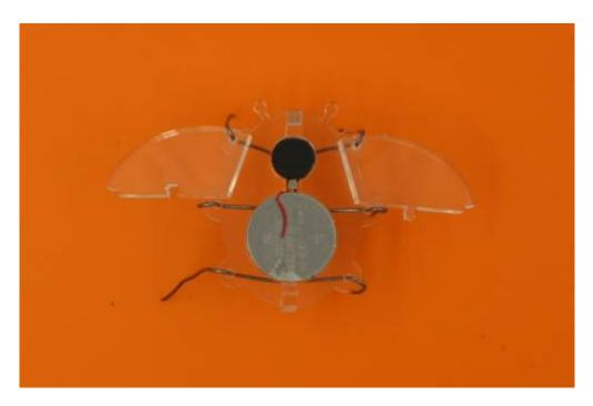
The remaining legs can now be attached, by inserting from the bottom as before. Try to get the length of the leg on each side the same.
