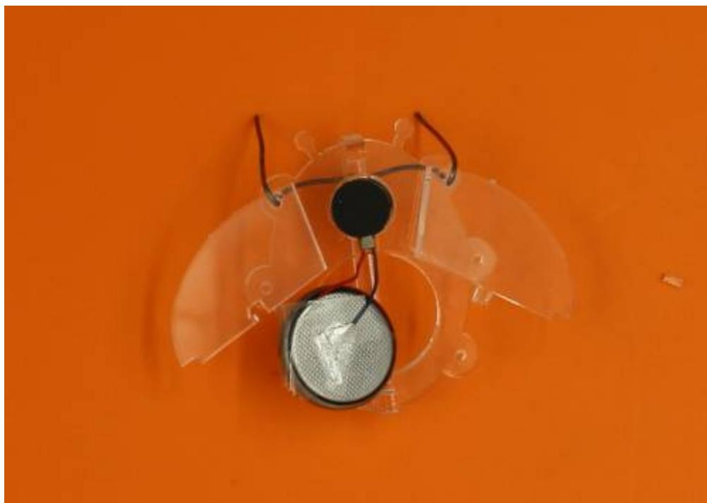
Place the battery in the larger hole in the body with the fixed wire underneath, and touch the red wire to the top face. The motor should begin to vibrate, showing the circuit is complete. Move the top wire
