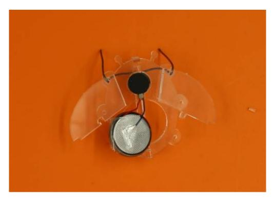
Place the battery in the larger hole in the body with the fixed wire underneath, and touch the red wire to the top face. The motor should begin to vibrate, showing the circuit is complete. Move the top wire
