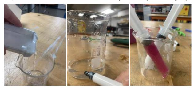
You can work out how much Silicone you will need to mix up by filling the container to the required height with water and then measuring this with a measuring cup. then halve this volume for Part A and Part B of the Silicone Preparation. With the small amounts required for badges i generally use 2 syringes to measure out Part A and Part B (2 cause you dont want the 2 parts mixing in the syringe (2)
