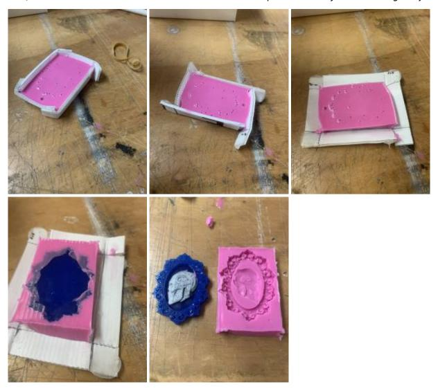
Curing will be complete in 20 mins. You'll be able to peel (clean)up any mess after the cure time.
