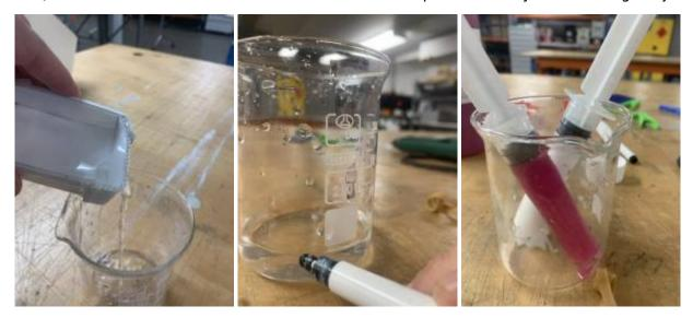
You can work out how much Silicone you will need to mix up by filling the container to the required height with water and then measuring this with a measuring cup. then halve this volume for Part A and Part B of the Silicone Preparation. With the small amounts required for badges i generally use 2 syringes to measure out Part A and Part B (2 cause you dont want the 2 parts mixing in the syringe (2))
