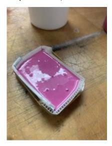
Mix Part A and B Thoroughly - mix untill all the Hot Pink and White streaks are mixed in. You have 2 minutes Mixing / "Pot Time" before the mix starts to cure. Curing will be complete in 20 mins. You'll be able to peel (clean)up any mess after the cure time.
