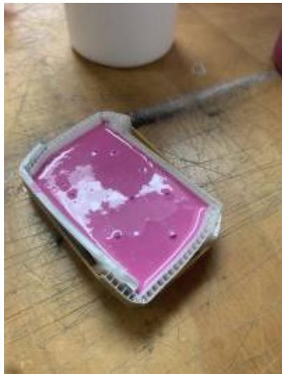
Mix Part A and B Thoroughly - mix until all the Hot Pink and White streaks are mixed in. You have 2 minutes Mixing / "Pot Time" before the mix starts to cure. Curing will be complete in 20 mins. You'll be able to peel (clean)up any mess after the cure time.
