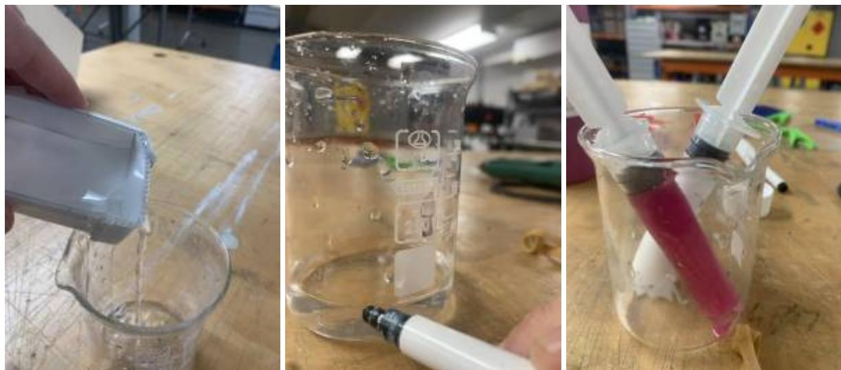
You can work out how much Silicone you will need to mix up by filling the container to the required height with water and then measuring this with a measuring cup. then halve this volume for Part A and Part B of the Silicone Preparation. With the small amounts required for badges i generally use 2 syringes to measure out Part A and Part B (2 cause you dont want the 2 parts mixing in the syringe 😊 )
