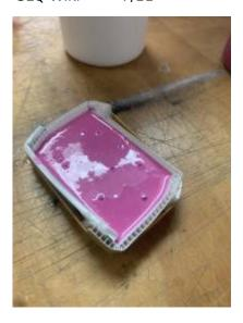
Mix Part A and B Thoroughly - mix untill all the Hot Pink and White streaks are mixed in. You have 2 minutes Mixing / "Pot Time" before the mix starts to cure. Curing will be complete in 20 mins. You'll be able to peel (clean)up any mess after the cure time.
