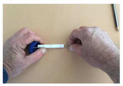
You will need a hook now to pull the rubber band through the centre of your hollow axle. Your unstretched rubber band should be hidden inside the axle, but the end of the hook will be available to finish the assembly.
