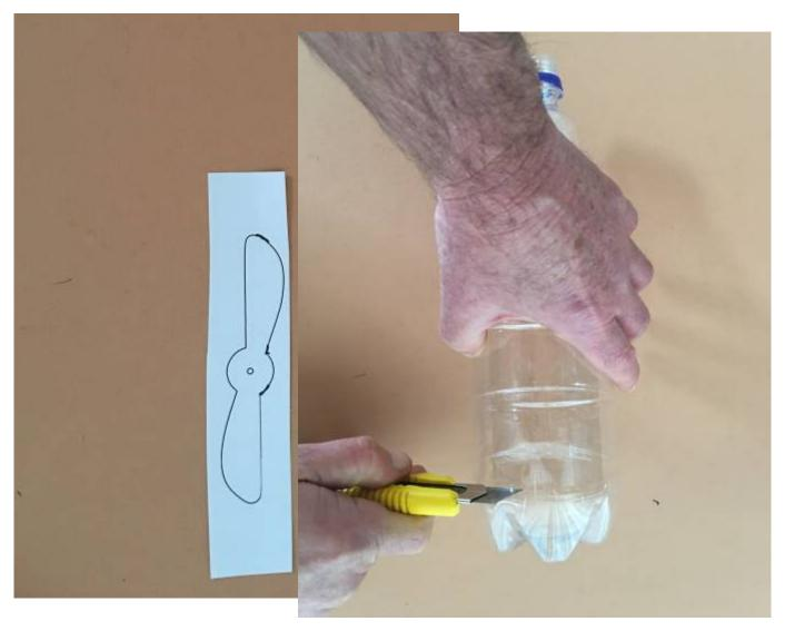
Now, cut a vertical strip of PET bottle a bit larger than the propeller template.
