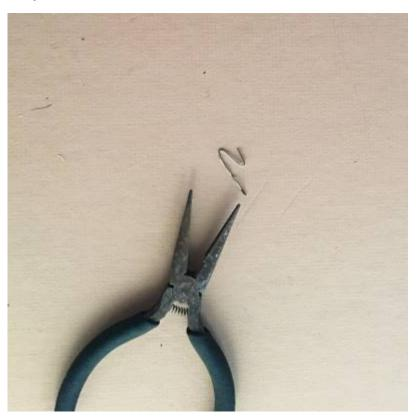
You will need a hook at the end of the straw to hold the rubber band, but it is best fixed in place later (alignment is important). Bend the tail hook into an Z-shape, as shown. The longer tail will slide inside the straw, to help keep the hook in place.
