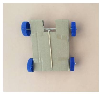
In this device the rubber band stores energy by stretching, rather than twisting, which means less power is available to make things happen. Because energy is only needed to turn an axle (rather than lift something into the air) this should not be a problem - unless you are attempting to set distance records. The basic approach can also be adapted to make a rubber powered paddle boat, if the wheels are replaced by paddles, and you make it out of some material more waterproof than cardboard.
