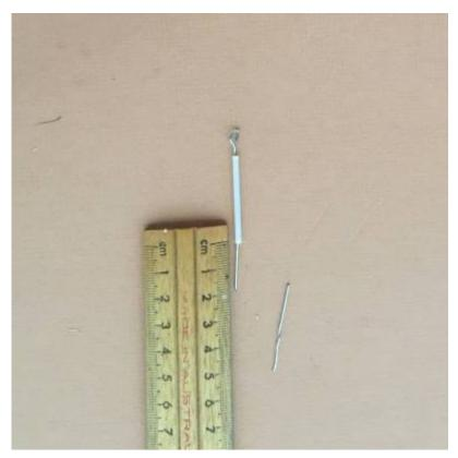
Slide the wire axle through the shaft bearing, and check it can rotate smoothly.
