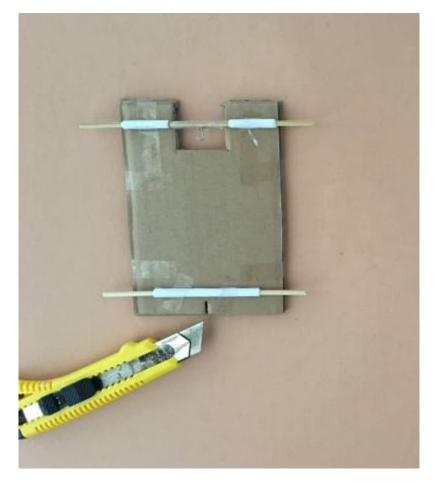
Mark the centre of the chassis at the front, and use a boxcutter or scissors to make a notch about 1cm long.
