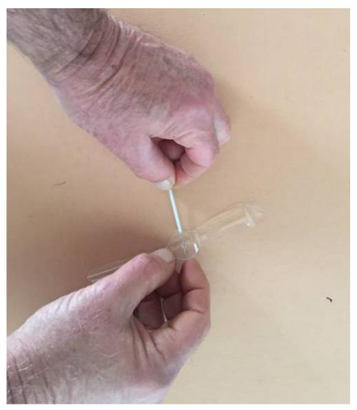
Slide the washer onto the propeller axle, and then the propeller. If your skewering has raised one side of these pieces, then place the two smooth sides together to minimise friction.
