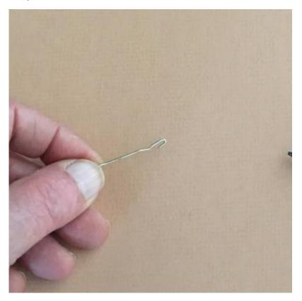
Straighten out a small paperclip, or find a piece of wire of a similar size. Steel wire will be best, since copper will more likely not stay bent under the rigours of use.
