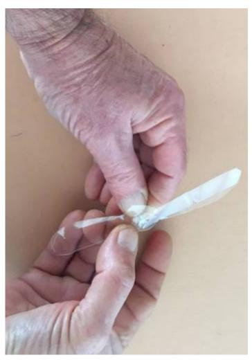
Push the propeller down the shaft, and use the pliers to bend the protruding shaft into a U-shape, with the open end of the U facing the propeller.
