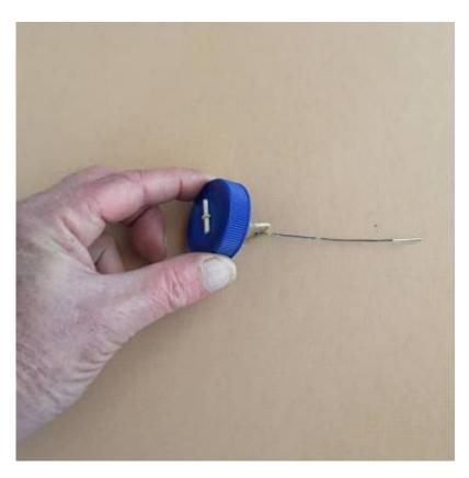
Insert the short stick through the loop of the rubber band on the outside of the wheel, and pull tight. This short stick will be held firmly against the wheel, and friction will transmit the force of the unwinding rubber band to the wheel.
