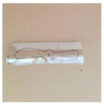
And then you can cut out the propeller. Use a metal skewer or something similar to make a hole at the centre of the propeller hub.
