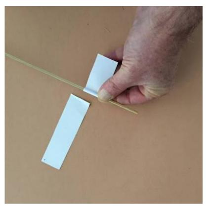
Use your chassis as a guide to make a strip of paper a bit narrower than the rear tabs and about 15cm long (half an A4 sheet is fine).
