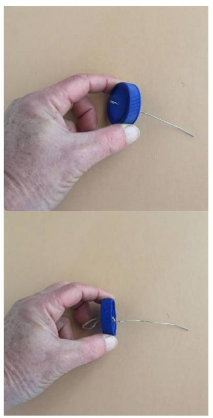
If you have made a large enough hole in the centre of the wheel, then you might be able to push the rubber band through. Otherwise, make a hook in the end of a piece of wire (a straightened paperclip will work well), and push the hook through the hole from the inside.
