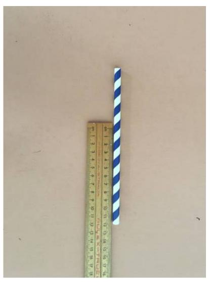
Cut the paper straw to a length of about 13cm. Scissors tend to crush the straw, and a boxcutter gently used like a saw will work better, especially if you work your way around the straw cutting one side at a time.
