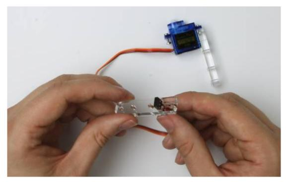
Take care to thread the electrical cord through the slot provided on the leg.
