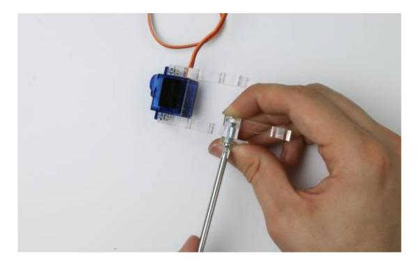
Fit the servo mount, with the servo arm facing inwards to the same leg.
