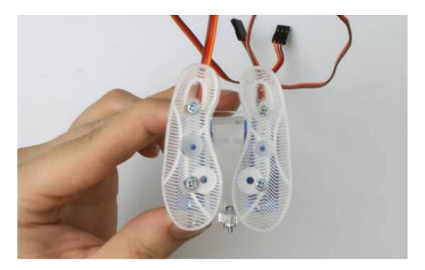
Now the center servo can be attached. Try to keep the frame as square as possible
