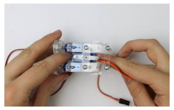
the battery holders boards and wires can then be taped to the counter-balance shaft.
