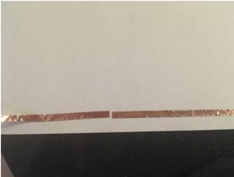
Fig 5. Leave a gap for the resistor
