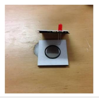
**3.** Bend the short contact of the LED up to almost flush with the E panel. Attach the F panel to the bottom of the E panel and ensure that the long contact of the LED slips inside the slot next to the coin battery. Bend the long contact up flush against the battery.
