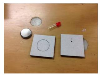
**2.** Slot the LED contacts into the E panel with the longer contact in the outer most hole and place the coin battery into the hole of the F panel (Negative side up).
