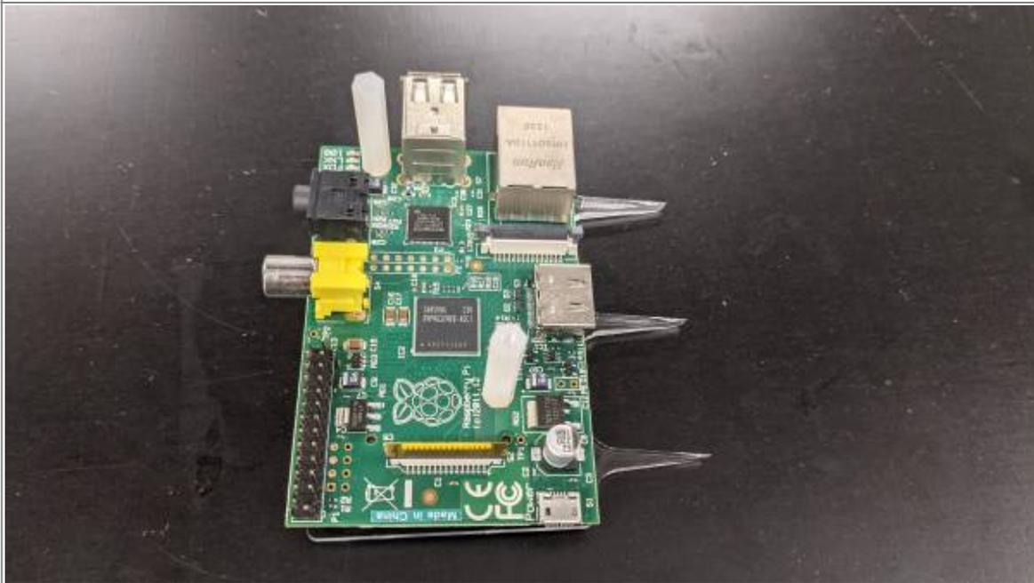
Attach the 2 standoffs to the screws on the front side
