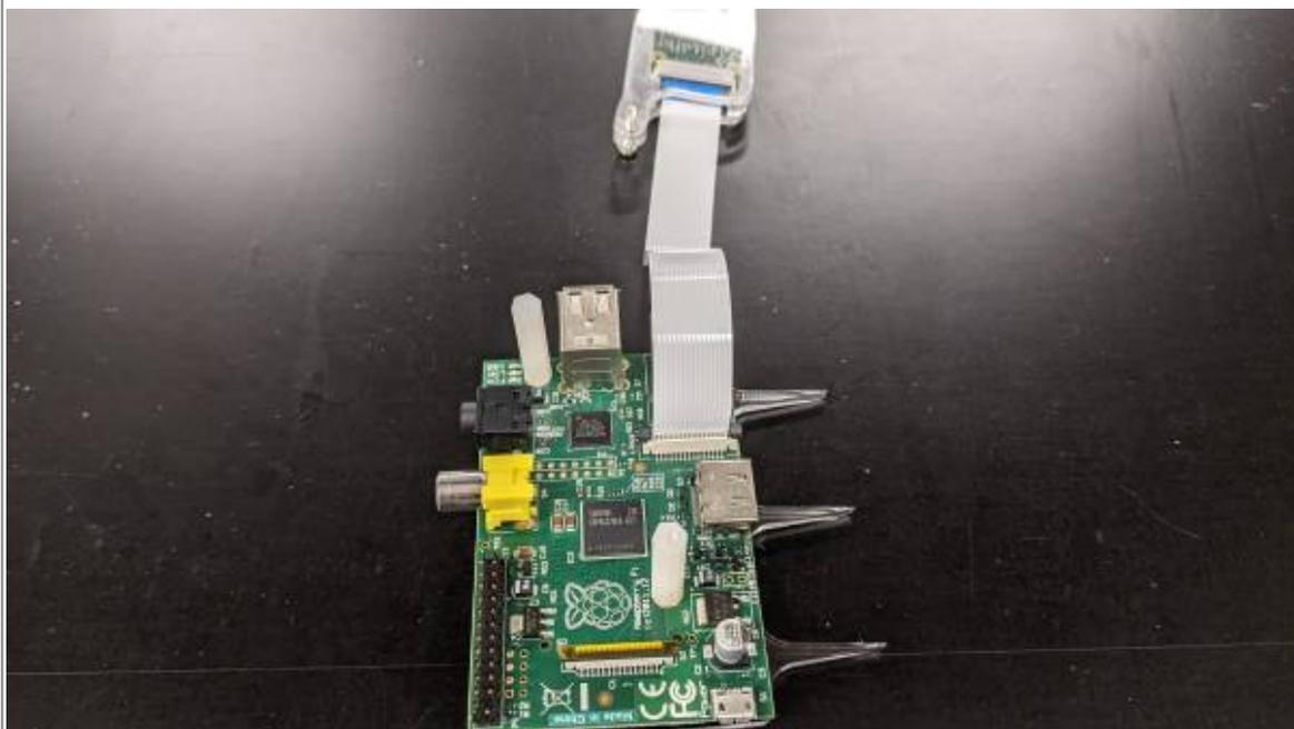
Plug in the camera by pulling the clip up, inserting the ribbon and pushing the clip back down to secure it. Ensure the ribbon cable is facing the correct direction, and you're plugging it into the camera port (not the display one).
