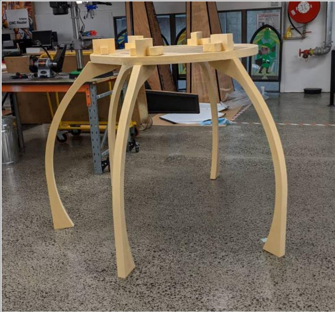
Cut the structure in 50mm XPS foam (note the 2 layers)
