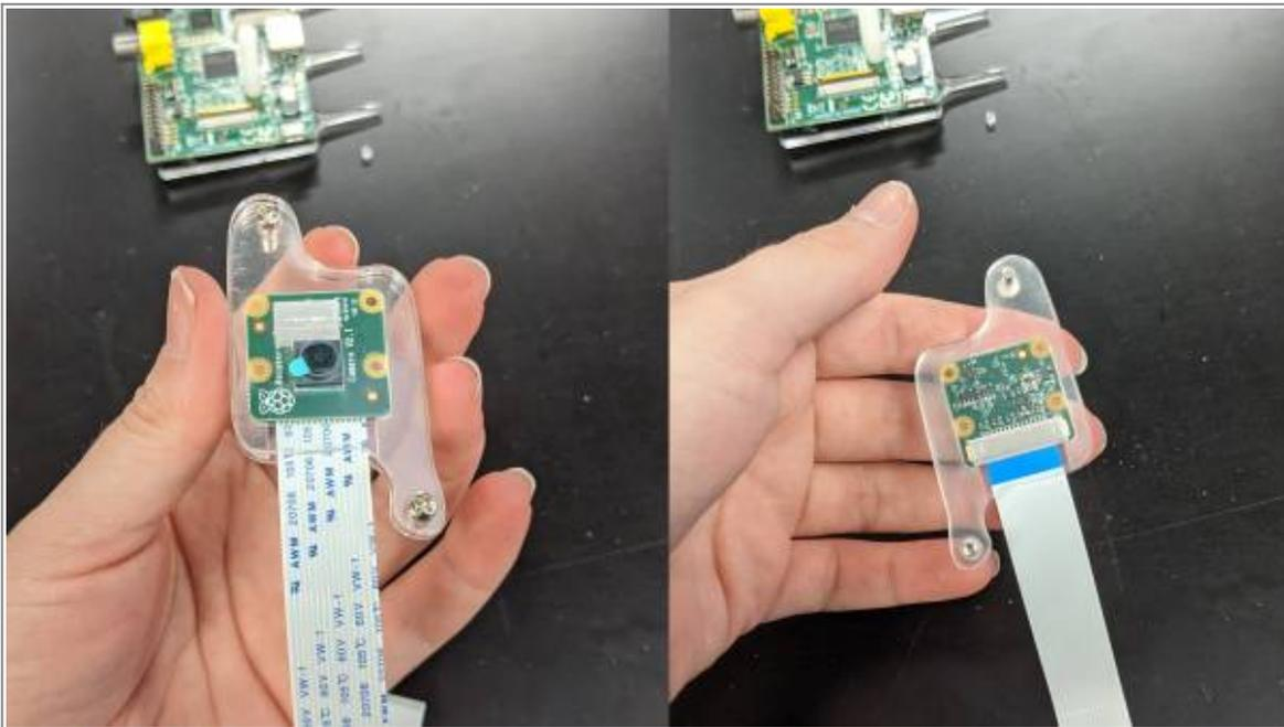
Assemble Camera mount, 3 layers of acrylic as per picture.
