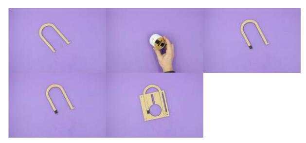
Once again, use a couple of skewers and work from the back to the front. The haps will be the middle layer (5th from both front and back). When all 9 layers are in place, snip off the skewers, once this is done we will remove the front layer for now. You can add a couple of rubber bands to keep everything together.
