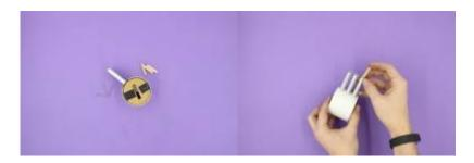
Grab the chamber support and put it over the chambers, the open end should be facing to the front of the plug/lock. It is important that you don't press the chambers into the actual plug, as it won't turn. Once the support is in place (you may need to hold it due to the tension from the springs), gently squeeze your plug housing and chambers into the hull, there should be some resistance so try wiggling in.
