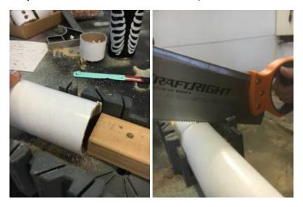
Again secure a timber stop in the mitre box measuring with a square, this time 50mm,
