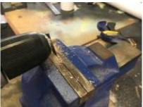
Set a hacksaw blade into a vice at about 45 deg. Set the dowel into battery drill chuck. cut your groove.
