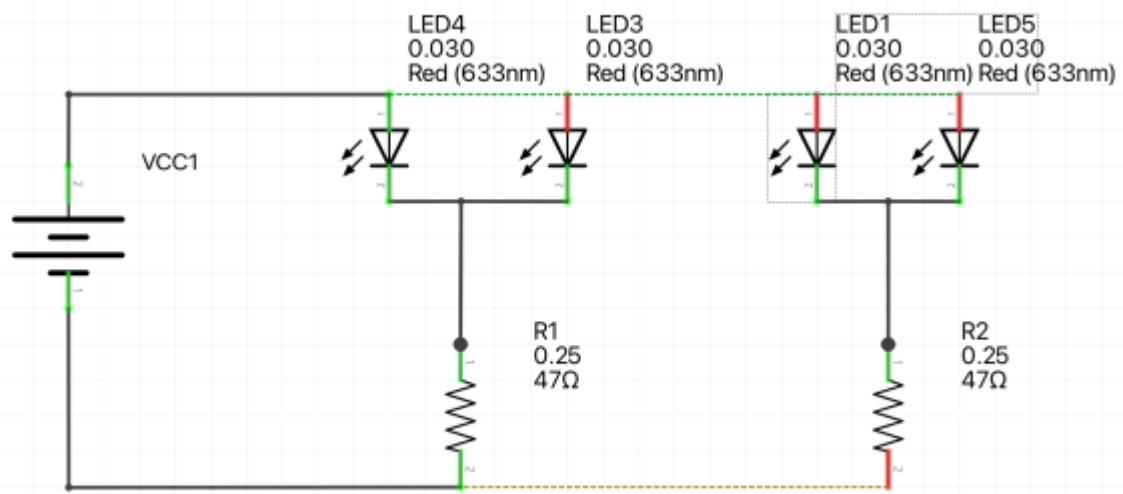
Positive accross the top and negative from the bottom via each of the resistors
