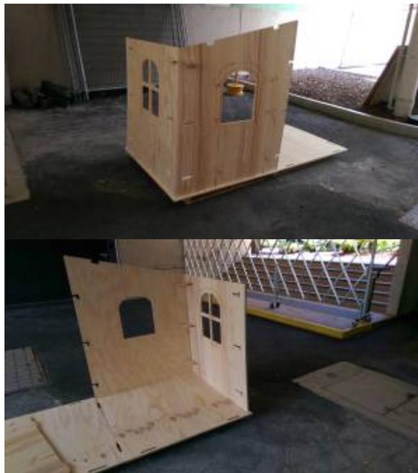
Then place the 3rd wall on one of the bases and assemble using the corner joinery install roof truss using 70x30 pine (4 required). Repeat for the other base.
