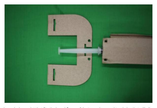
The claw yoke has a slot that fits the barrel flange of the top syringe, and two holes that will align with holes in the top of the handle.
