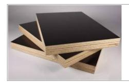
Formply—an exterior-grade plywood faced on both sides with resinimpregnated paper. The smooth faces release easily from the cast concrete.
