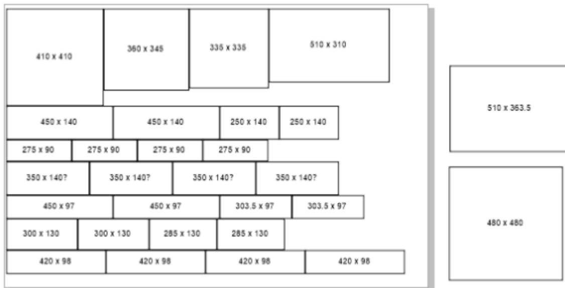
*Sheet layout for cutting workshop mould box sides and bases from 1800 x 1200mm panel*
