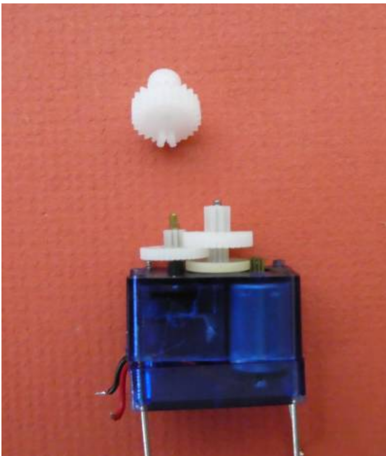
Gently slide the gear off the shaft.
