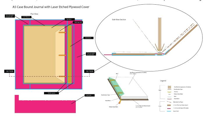
This is mostly 1:1 scale so drawings can be used to laser cut guides, templates and the covers. An Al file is in the downloads at the bottom of the page.
