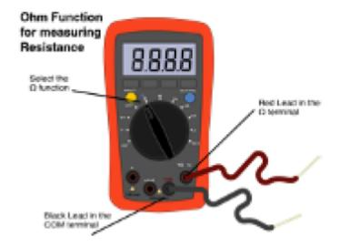
Select the continuety setting by • selecting Ohm on the Dial  $\Omega$  • And use the blue button in the image above to select the continuity setting  $\delta$
