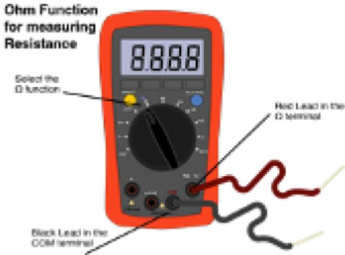
Select the continuity setting by • selecting Ohm on the Dial  $\Omega$  • And use the blue button in the image above to select the continuity setting 📡
