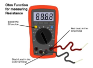
Select the continuety setting by • selecting Ohm on the Dial  $\Omega$  • And use the blue button in the image above to select the continuity setting  $\delta$
