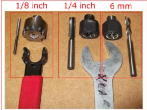
• While pressing down yellow 'Spindle Lock' button, loosen collet to remove previous tooling.
