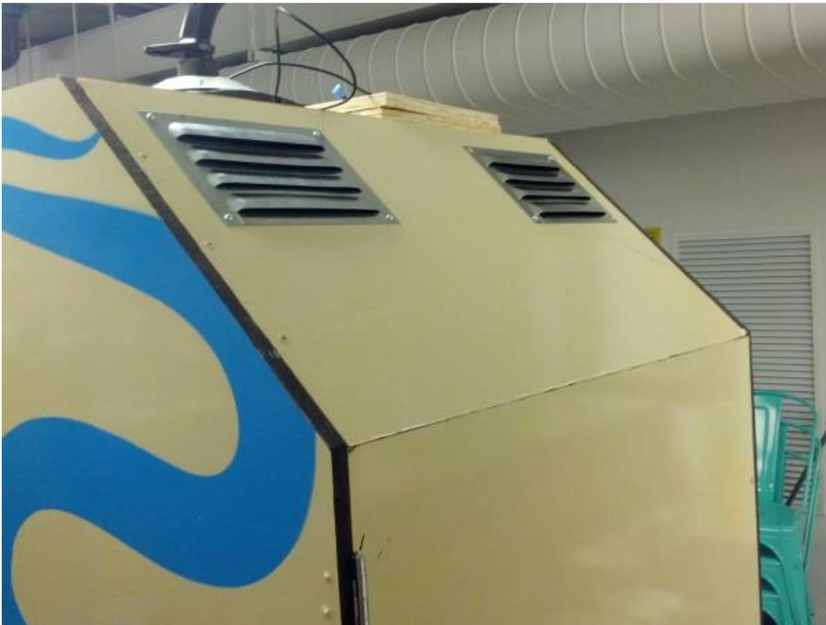
Once it was realised that the cabinet would end up being installed in open public areas and games started to be donated, a simple lock was installed. As the cabinet is just screwed together anyway, something that would prevent opening without tools was chosen as adequate.
