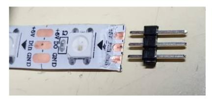
• Tin contacts to ensure they are clean, tin short end of connector. Solder connector in place. Using a socket of some kind helps keep them aligned.
