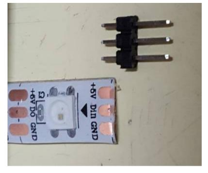
• Some waterproof strips have a cover, cut and peel back the last few mm to expose bare copper.
