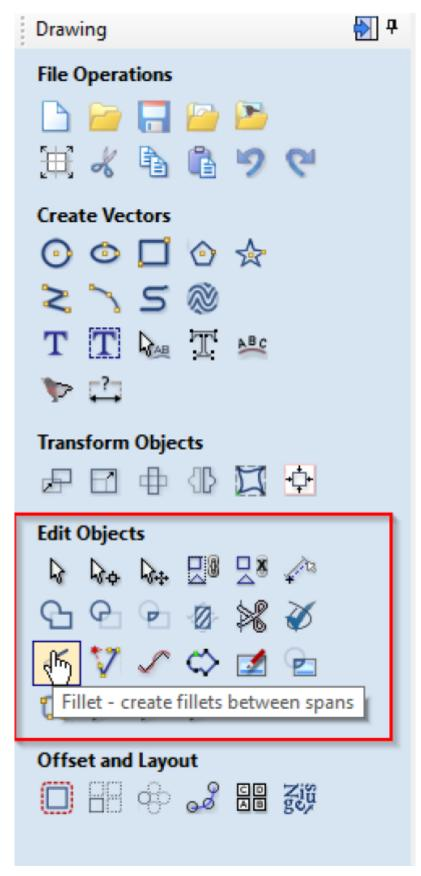
And set the fillet/tool radius to 1/2 your tool diameter, selecting **dogbone** as the fillet type.
