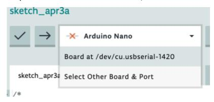
In the search field on the left under *BOARDS* make sure you select the regular Arduino Nano (there are other variations). The COM *PORT* should already be correct, if it isn't you can change it to what was displayed in the Device Manager. Finally we need to select the *FLAVOURS*, select ATmega328P (Old Bootloader). Our particular board uses the old bootloader variant. Press OK once all these settings are correct.
