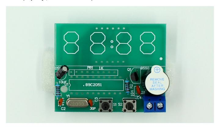
Integrated circuit (U1). Align notch with symbol on PCB.
