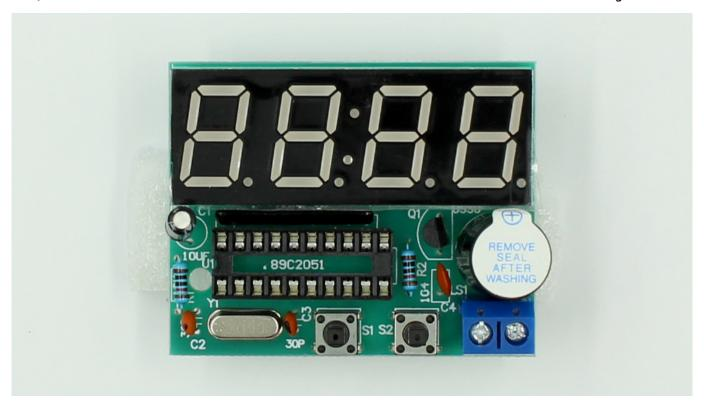
Insert integrated chip, bend legs accordingly
