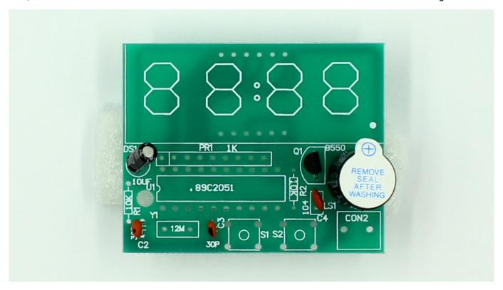
Resistors (R1, R2). Go in either way.
