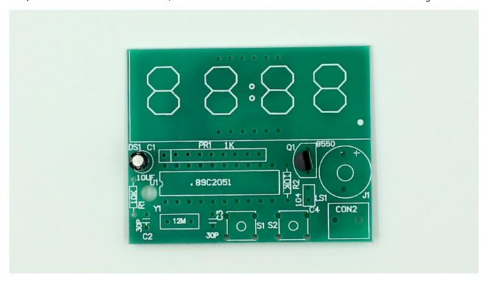
Piezo Buzzer (8550). Match up positive side with marks on board.
