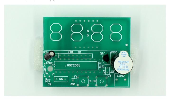
Capacitors, Large (C4), Small (C2,C3). Legs go in either way.
