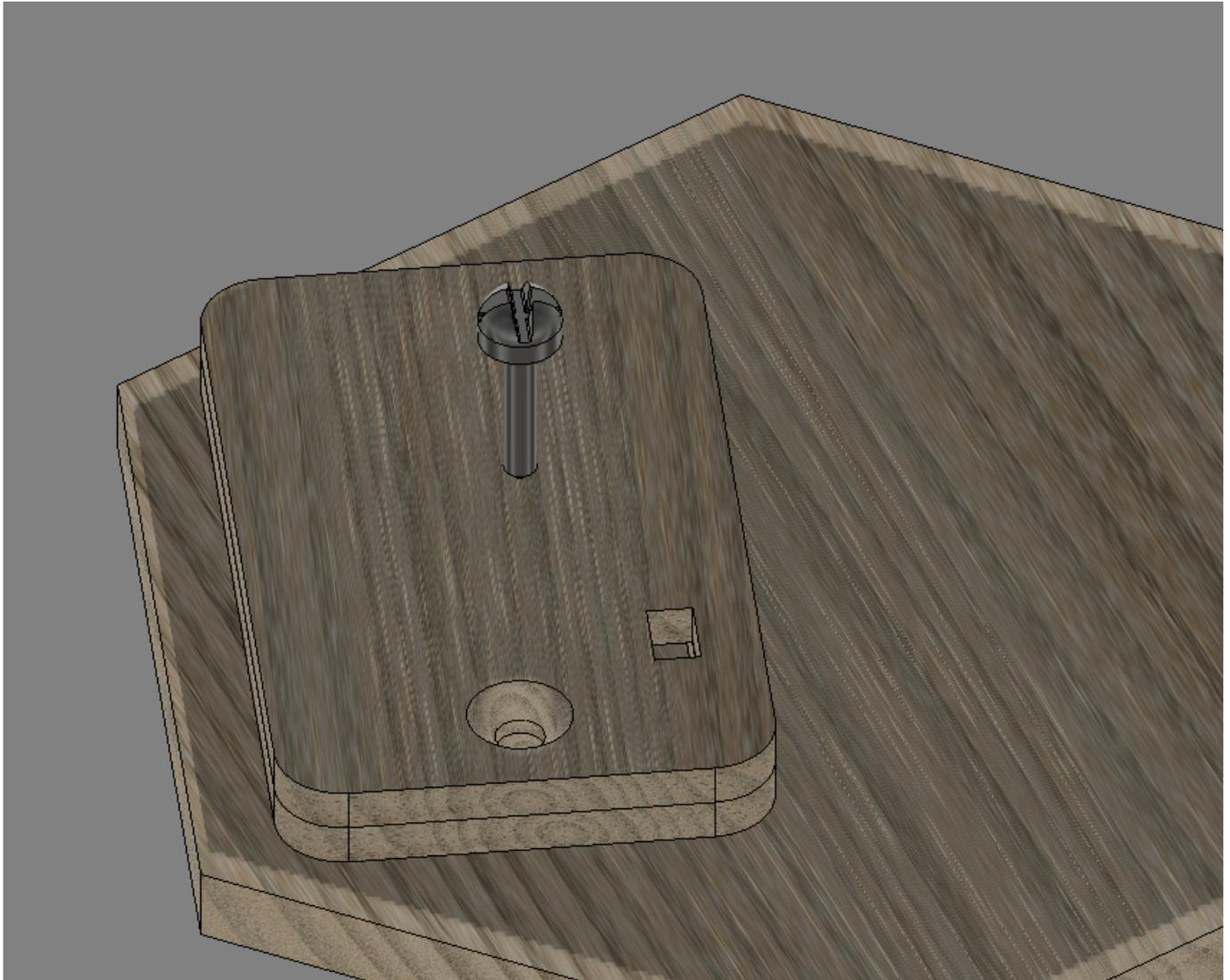
Insert **Screw (part)** from back to front and screw on nut.
