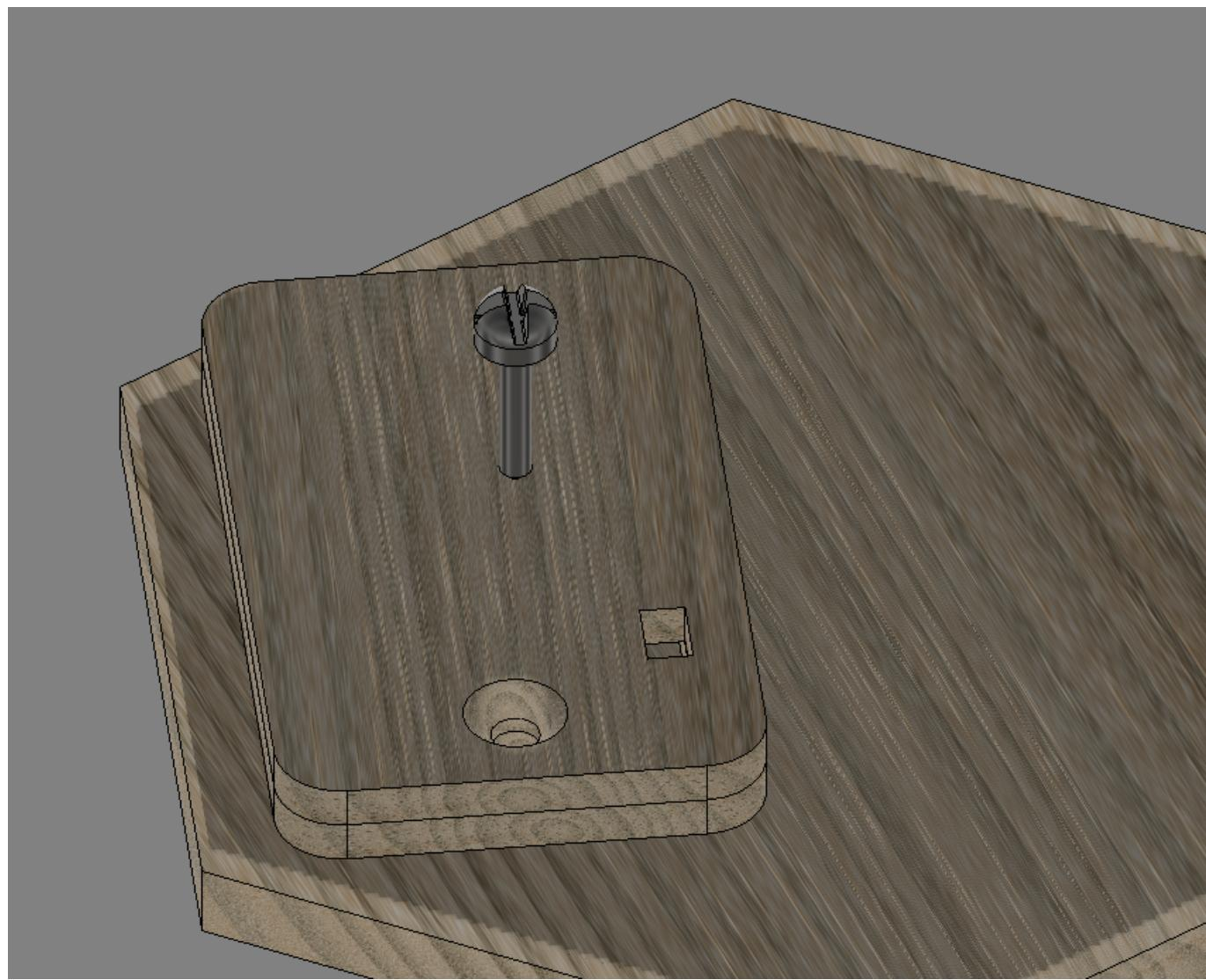
Insert **Screw (part)** from back to front and screw on nut.
