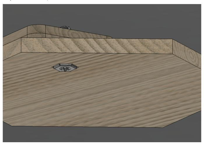
Tighten Nut and bolt using Phillips head screwdriver and adjustable spanner.
