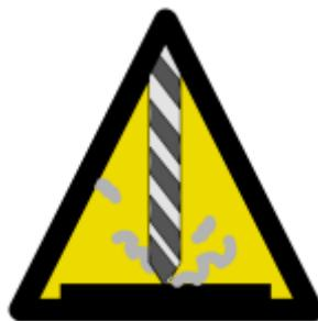
Also any time you are using a spinning blade or tool you could be creating friction... **Be careful of hot tools and keep track of where your hot swarf ends up**
