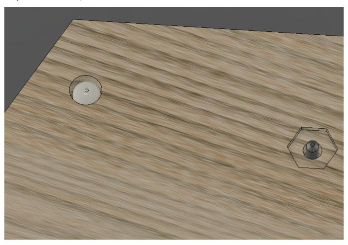
Turn the badge over again so it is face down and insert the Cell (battery) with the positive (+) up.
