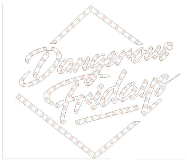
Next is time to remove any small curves - Pull up the Fill/Scallop/Chamfer docker. The Multicam guys say 5mm radius is fine - but I'm going to set 10 mm 'cause I ain't breaking the knife.
