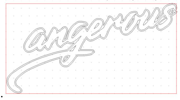
• Resize all parts using the 'precision input centre' (F2) to .95 of original proportions.(do a quick calculation to see if we've stuffed our line thickness...15 \* .95 = 14.35.. should be fine)
