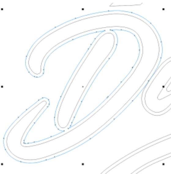
Where this weld has resulted in a sharp corner, I've filleted again to smooth it out.
