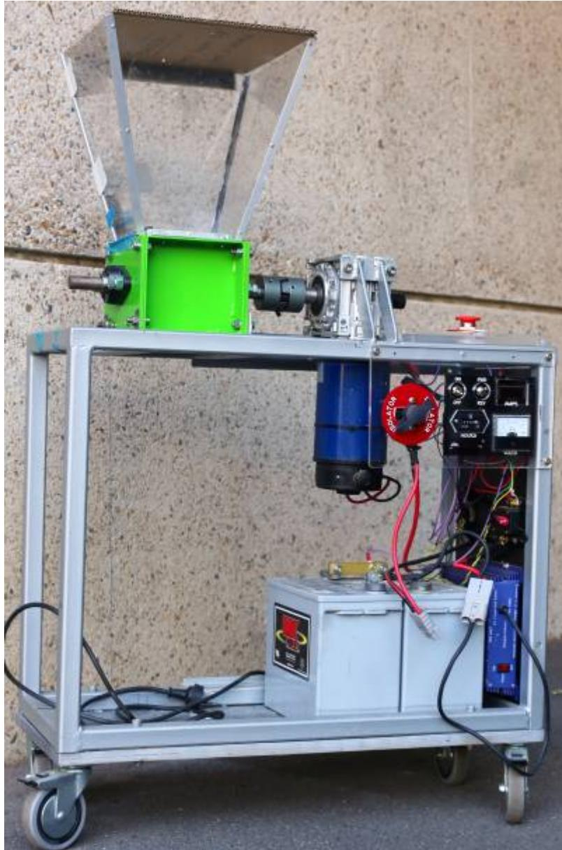
Shredder components were laser cut by external service providers according to the design files available from the <https://preciousplastic.com/en/> website, with the following modifications:
