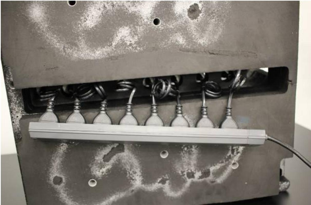
Wedge the powerboard into the bottom of the foam - make sure the powerboard lead is fed up through the hole.
