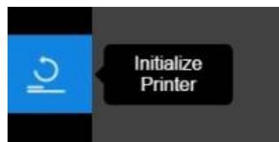
The first step that needs to be undertaken before printing is to initialize the printer. That can be done by pressing the initialize button on the left hand side menu. Most other options/button will be grayed out until this step has been completed. The initialization should only take a minute or so and you will
