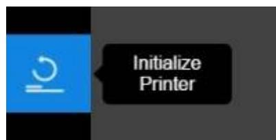
The first step that needs to be undertaken before printing is to initialize the printer. That can be done by pressing the initialize button on the left hand side menu. Most other options/button will be grayed out until this step has been completed. The initialization should only take a minute or so and you will
