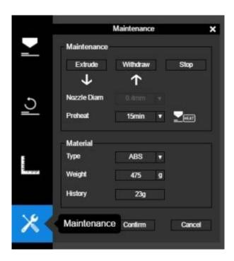
Before each print you should make sure that the filament is extruding properly. This can be done by going to the maintenance menu and clicking "Extrude". If you want to make changes to the material
