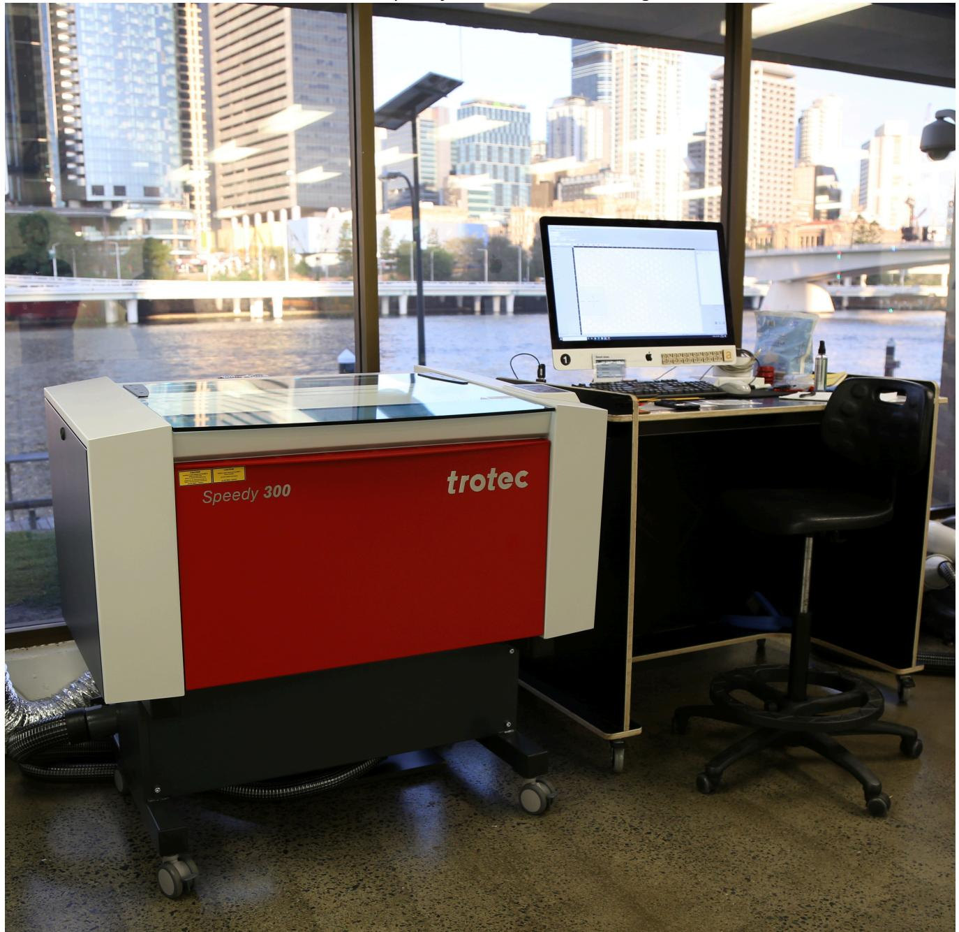
The Trotec Speedy 300 is suitable for laser engraving and cutting of wood, plastics, leather, paper and many other materials. The materials we use in-house are plywood, acrylic, boxboard, polypropylene and paper.
