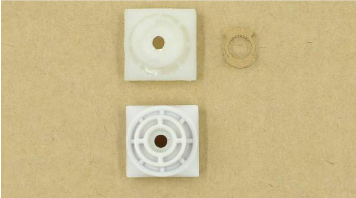
And here is how the acrylic gear meshes with the spur gear.
