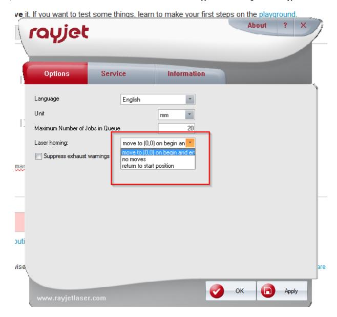
Change the homing to no moves if you are using nuts to hold down a warped material.
