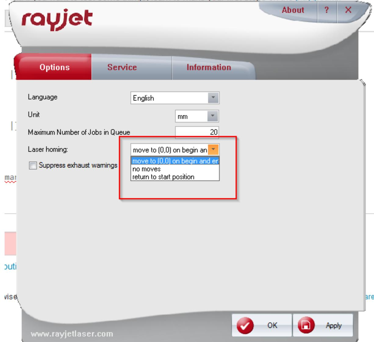
Change the homing to no moves if you are using nuts to hold down a warped material.
