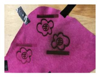
The first test (Far Right) was etched at the same settings as Balsa 40% power 95% speed- this was too much (sooty and could not see the gradation in the contrast bar. 2nd test (Far left) was 20% power 95% speed 3rd test (top) was 27% power 95% speed - I'd recomend somewhere between these last 2 settings
