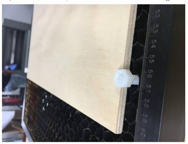
We fed the bolts ( with a metal spring washer) up through the honeycomb and clamped the timber down with the corner of the nut. When I get around to it I'll make some acrylic washers/ clamps to grab the timber in a more secure way. The timber popped up when it was cut but at least it was cut etched and then flat.
