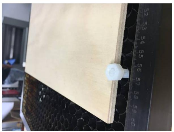
We fed the bolts ( with a metal spring washer) up through the honeycomb and clamped the timber down with the corner of the nut. When I get around to it I'll make some acrylic washers/ clamps to grab the timber in a more secure way. The timber popped up when it was cut but at least it was cut etched and then flat.
