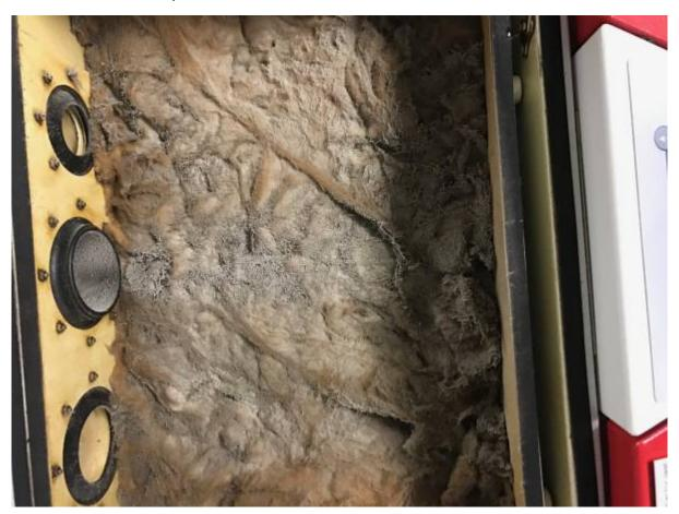
The filter had not been cleaned in over two months. The pre-filter was caked solid with materials and the HEPA component of the filter system blew out. Would suggest that this as a direct result of the lack of cleaning and maintenance on the system and that this shortened the life of the filter.
