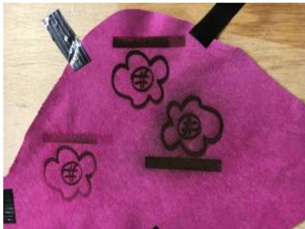
The first test (Far Right) was etched at the same settings as Balsa 40% power 95% speed- this was too much (sooty and could not see the gradation in the contrast bar. 2nd test (Far left) was 20% power 95% speed 3rd test (top) was 27% power 95% speed - I'd recomend somewhere between these last 2 settings
