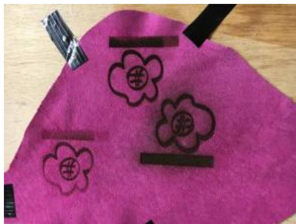
The first test (Far Right) was etched at the same settings as Balsa 40% power 95% speed- this was too much (sooty and could not see the gradation in the contrast bar. 2nd test (Far left) was 20% power 95% speed 3rd test (top) was 27% power 95% speed - I'd recommend somewhere between these last 2 settings
