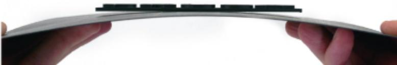
If you continue to experience difficulty with removing a printed object, you can gently introduce a non-metal flat spatula with rounded corners underneath the object to prise it free without damaging the PEI.
