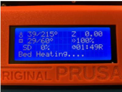
The printer will automatically commence heating the nozzle and the bed to the correct temperatures for the chosen filament; printing will start when the target temperatures are reached. This can take several minutes.
