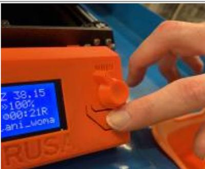
For a catastrophic failure press the **Reset (X) button**. This will abort the job and force a full reset of the printer.
