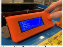
Using the Control knob, navigate to and select your file on the SD card (rotate knob to scroll, push to select). The last file saved to the card will appear at the top of the list.
