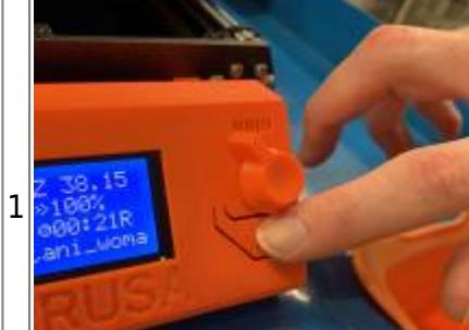
For a catastrophic failure press the **Reset (X) button**. This will abort the job and force a full reset of the printer.
