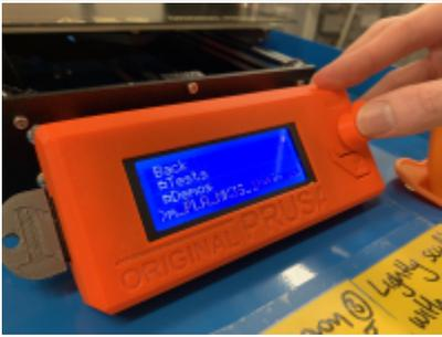
Using the Control knob, navigate to and select your file on the SD card (rotate knob to scroll, push to select). The last file saved to the card will appear at the top of the list.
