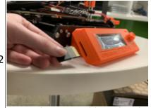
Insert the SD card into the slot on the side of the LCD screen assembly
