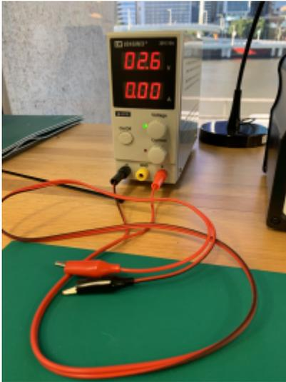
Digital display, analogue control, switch-mode based bench supply.
