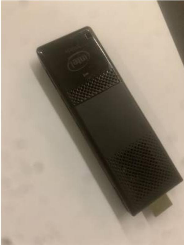
Compute Stick is a portable PC that's great for signage. Here's some instructions for setting up a video to autoplay MP4 off a USB stick on the digital signage screens on level one of the edge (or any other HDMI-equipped screen for that matter)
