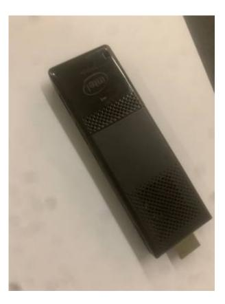
Compute Stick is a portable PC thats great for signage. Here's some instructions for setting up a video to autoplay MP4 off a usb stick on the digital signage screens on level one of the edge( or any other HDMI equiped screen for that matter)
