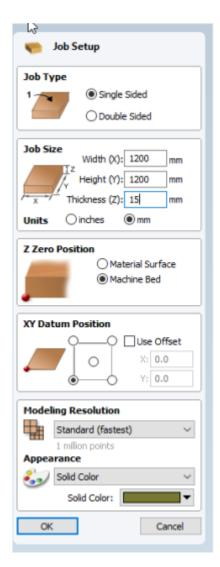
Make sure your material dimensions match your Job dimensions. For the inductions we use use a 2400x1200x17mm sheet. Measure all dimensions on the sheet!
