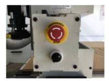
This can be activated to bring the machine to an immediate stop in an emergency.
