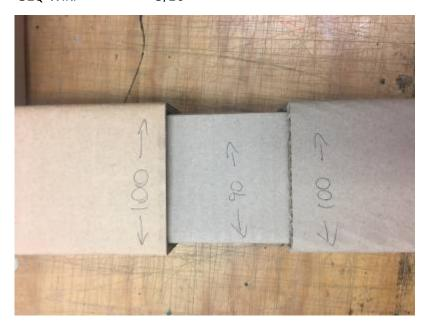
Glue one end in first, and apply glue to the exposed 90mm part, then push the other 100mm beam on.
