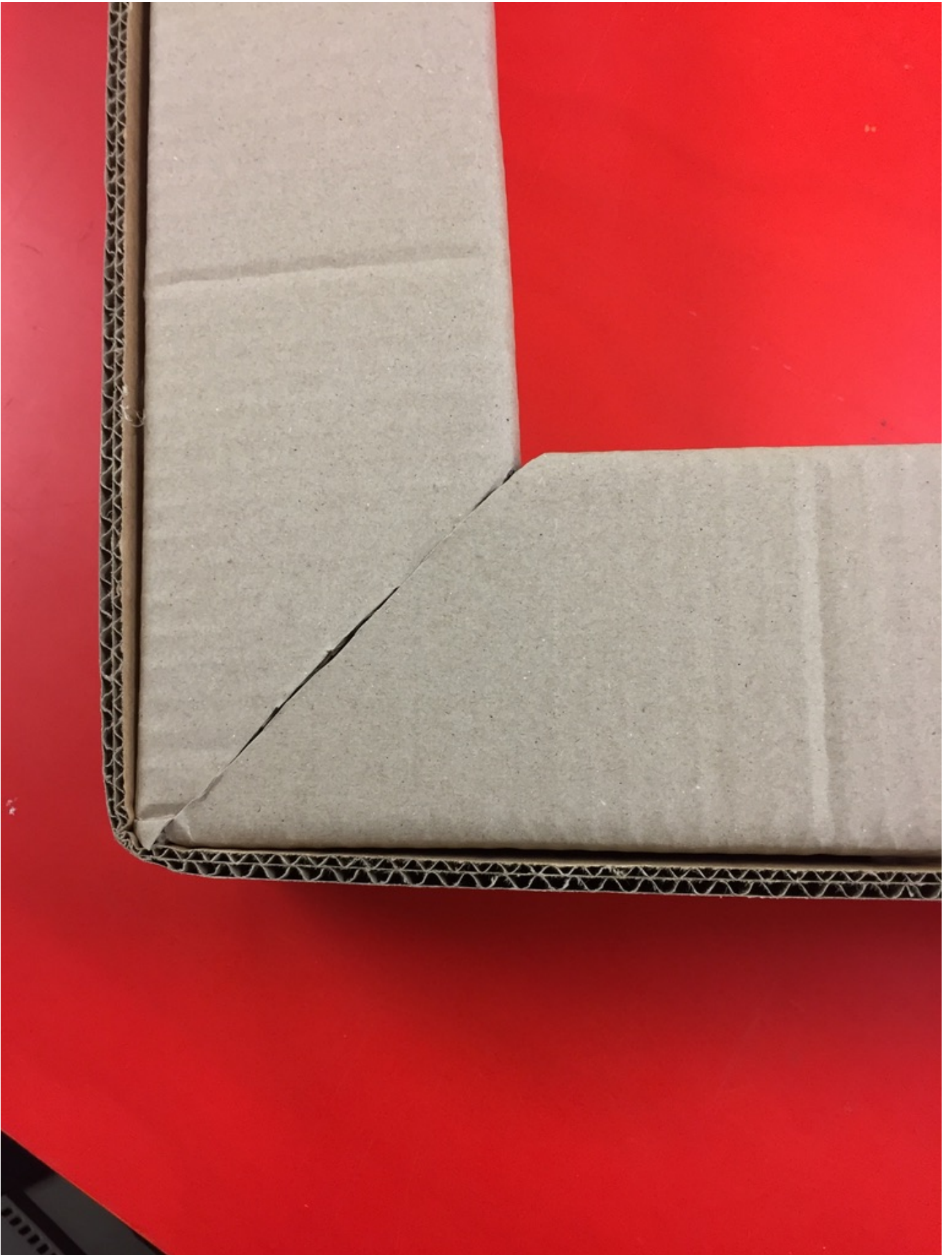
You can glue a piece of cardboard over the outside of the joint to secure it or refrain from cutting the
