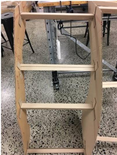
Z-element slots were used to keep ribs
