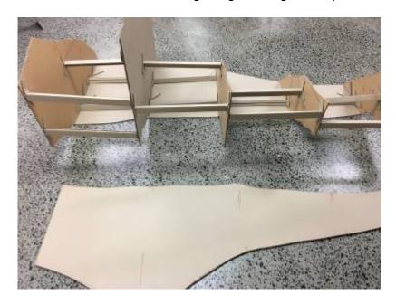
The same process was used to mark out and cut the centre join plate needed for this module. The lower LHS module did not have a central join plate because the shark is hollow.
