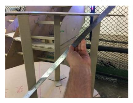
A rough measurement was made while the sections were held in place, and a single strip brace was made to help support the hanging piece.
