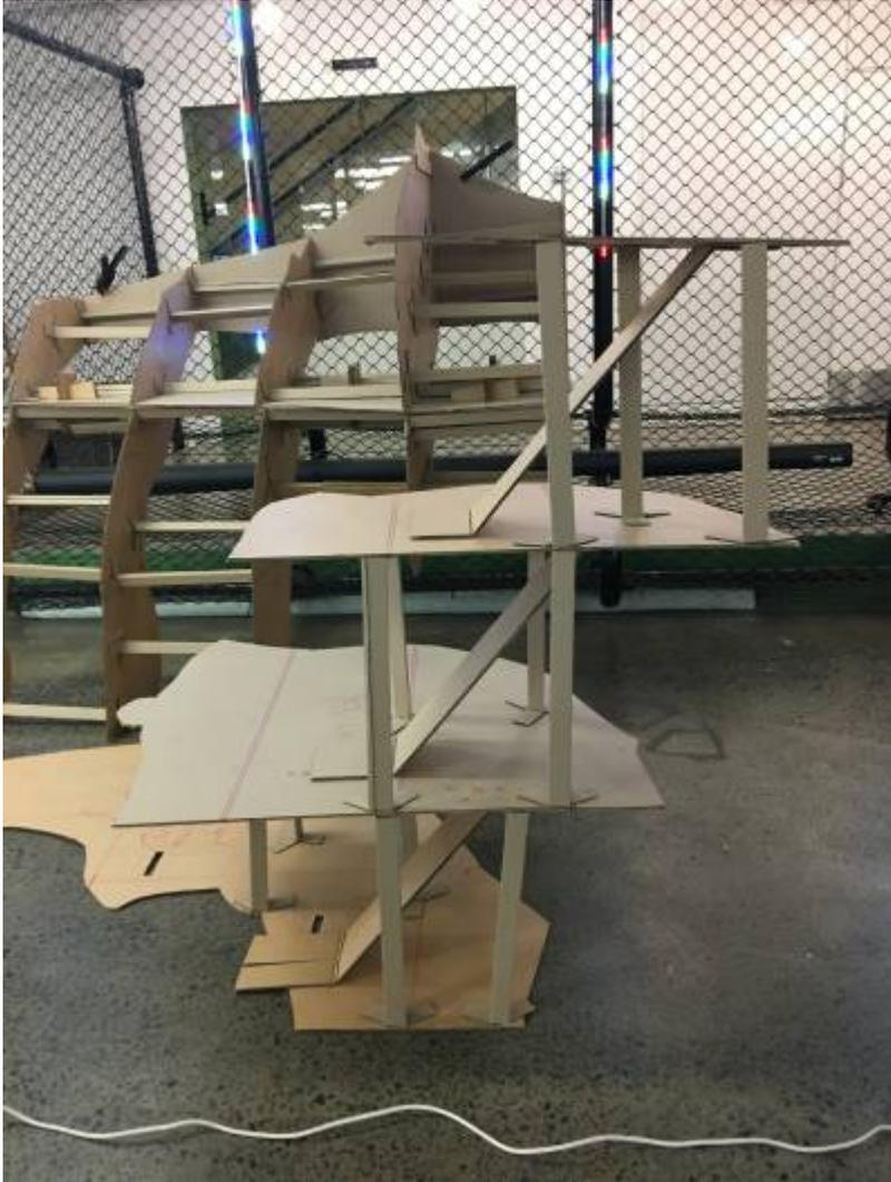
This approach was repeated for the other Y-elements in this module. (The side of this construct facing the viewer will be the vertical centre join plate - the braces run from high on the hanging piece, to low on the support piece)
