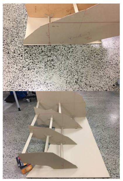
Place the module straight side down on a single sheet of cardboard. If possible, use edges of the plate sheet to align the pieces. Propping was necessary to get all the straight edges flat on the plate.
