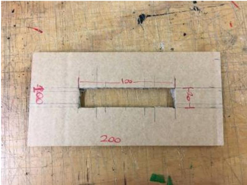
First, make a connector by gluing 3 pieces of double ply cardboard together (6mm thick) with the dimensions shown. This can also be used as a jig to draw the slots onto the sheets as required.
