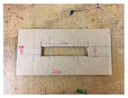
First, make a connector by gluing 3 pieces of double ply cardboard together (6mm thick) with the dimensions shown. This can also be used as a jig to draw the slots onto the sheets as required.
