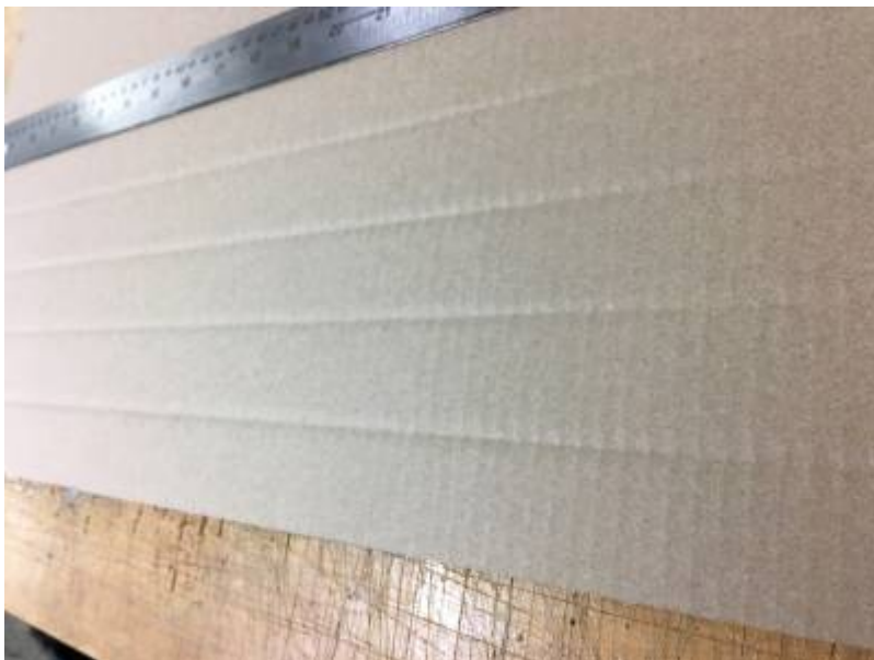
Scoring completed - note that cardboard is NOT broken along the score. This maintains strength.
