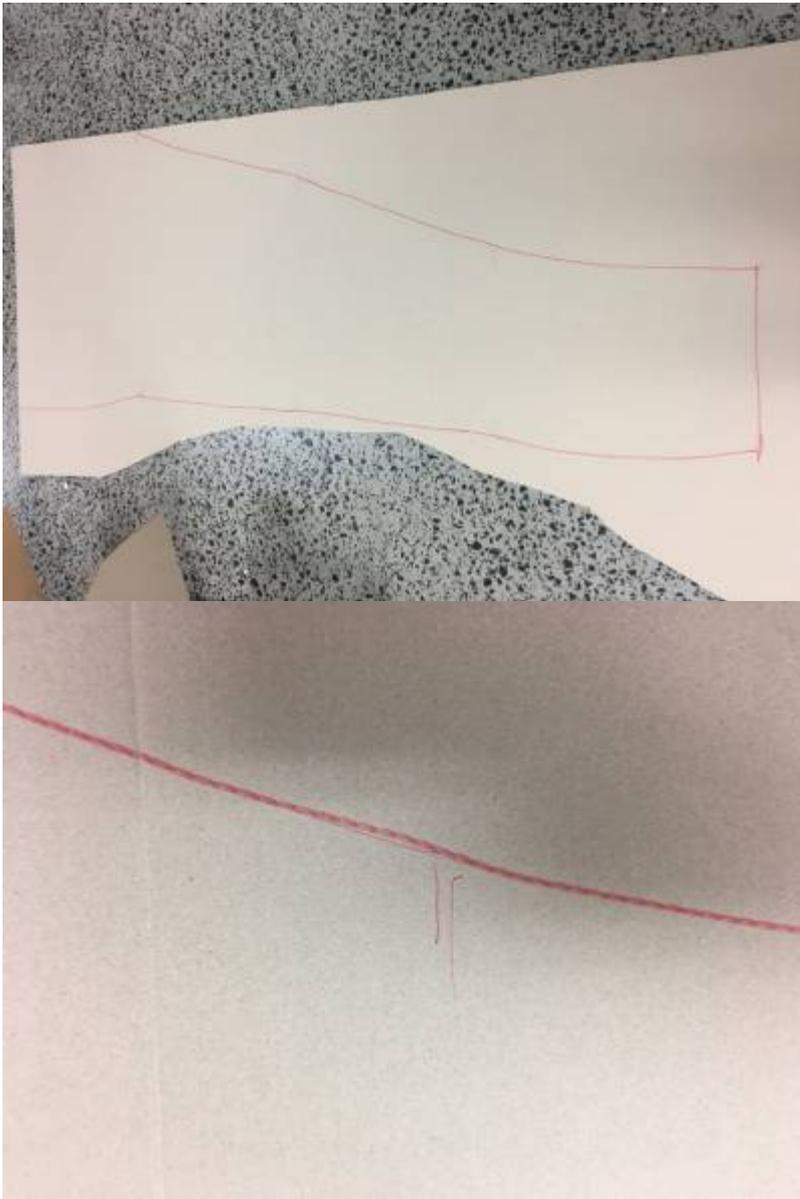
Trace the outline of the module onto the plate, marking where the Y segments sit for easier assembly later. Cut around the outline, and the plate is ready.
