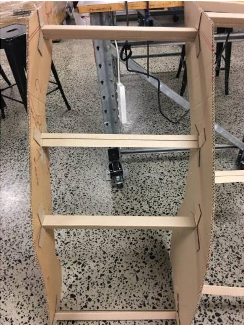
Z-element slots were used to keep ribs horizontal, and vertical registration lines to keep them parallel.
