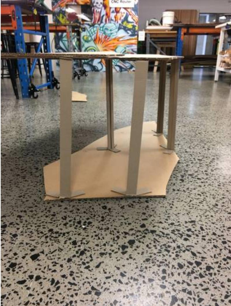
As before, use registration marks and ribs to join the Y-segments together. Keeping ribs perpendicular was again a problem - having registration marks that transfer a common cartesian grid to both sides of the elements would be a good idea.
