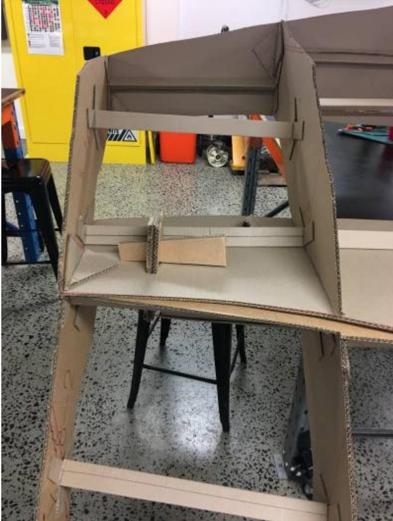
Holes were cut through both join plates, wedges prepared and added as shown. Note the holes were aligned so the wedges ran parallel to the ribs to avoid interference.
