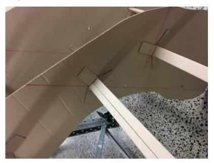
Aligning ribs to keep them horizontal and parallel to the centre axis of the model was an issue (another reason for lots of registration marks).
