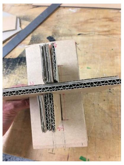
Push a wedge in from either side as shown, and tap them down to make a solid connection. Keep the sheets perpendicular to the connector as you go.
