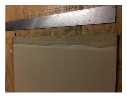
After measuring, a flap was cut, and worked to make a curved surface following the lines of the Yelements. This means the flap might not always be a square piece. The edge where the flap is attached to the skeleton was crushed from both sides, to make a more flexible join. SLQ Wiki 50/52 Reflective Practise
