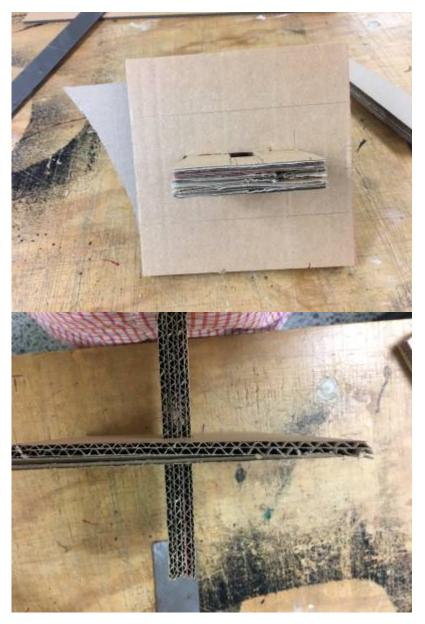
Cut two 100 x 20 holes in the sheets to be joined, and hold them together so the holes align. Push the connector through.
