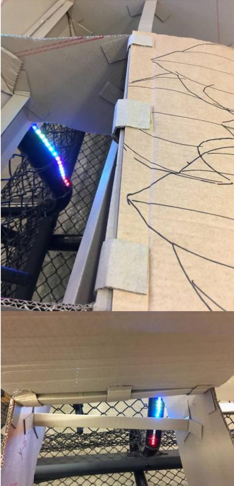
A few 50mm wide strips were cut to make the hinge, and thoroughly worked (crushed and bent over the edge of a bench) to make them almost circular. These pieces need to be long enough to reach loosely around the rib, with about 50mm at either end for gluing to the skin.
