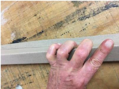
Run a bead of glue along the glue tab
