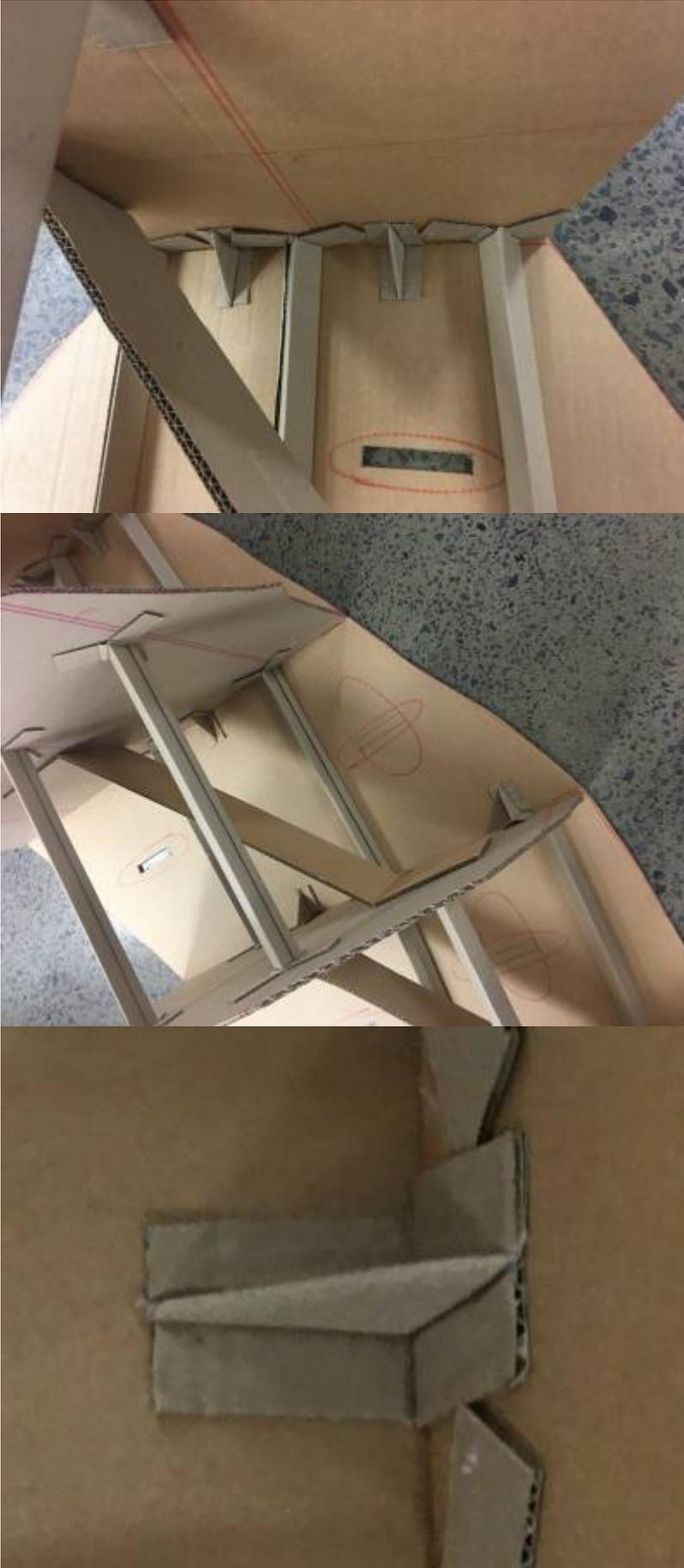
Attach the supports by adding glue to the underside of the margin flaps, and pressing it firmly into the angle between the two sheets you are joining. You can see why these supports were made small - there is not a lot of space between ribs in places.
