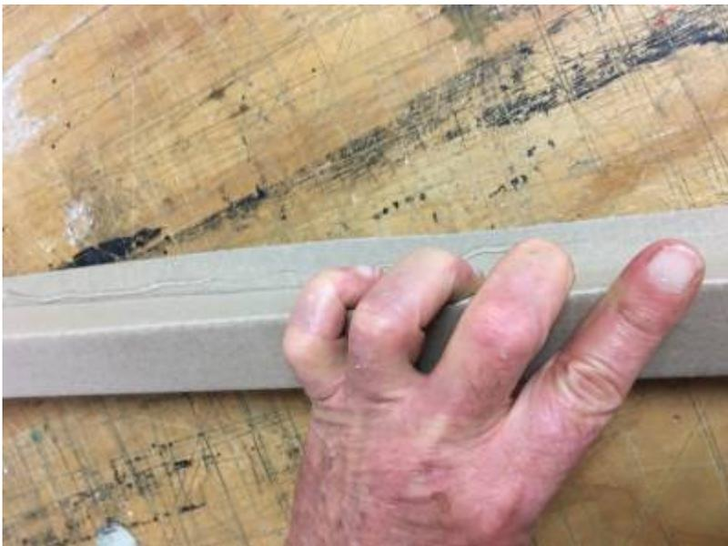
Run a bead of glue along the glue tab (both ends and a bit in the middle is usually enough).
