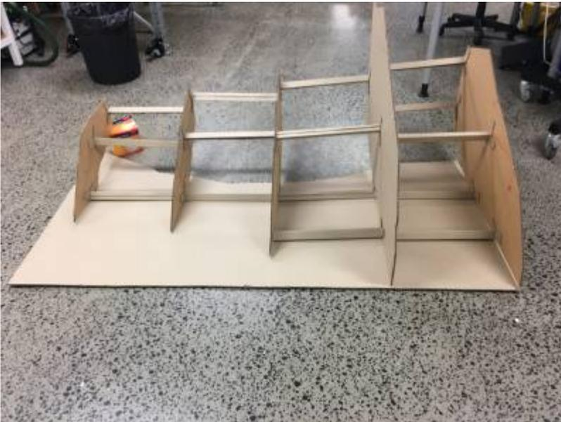
The finished section set out on a single sheet of cardboard to trace and cut the joining plate.
