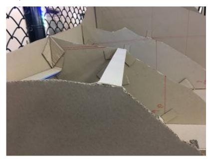
First, a triangular rib was put between two of the Y-elements that open to a cavity containing wedges. The rib was placed with a surface flush with the hinge line.
