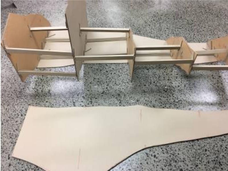
The same process was used to mark out and cut the centre join plate needed for this module. The lower LHS module did not have a central join plate because the shark is hollow.
