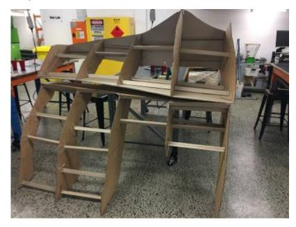
The registration marks were used to align the ends of the two module, but warping meant a good horizontal alignment was not achieved.
