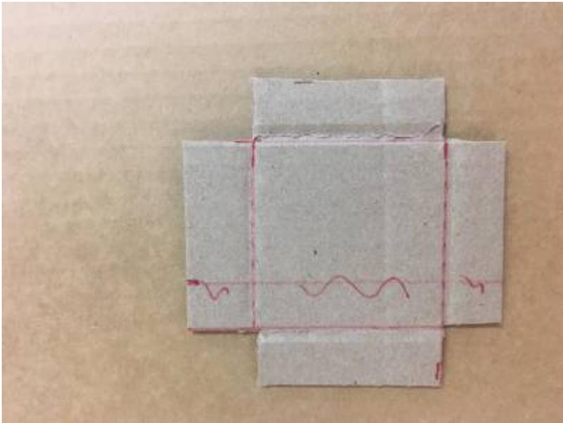
Flip the piece over, and make a diagonal score along the back. On the front, score along the margin lines
