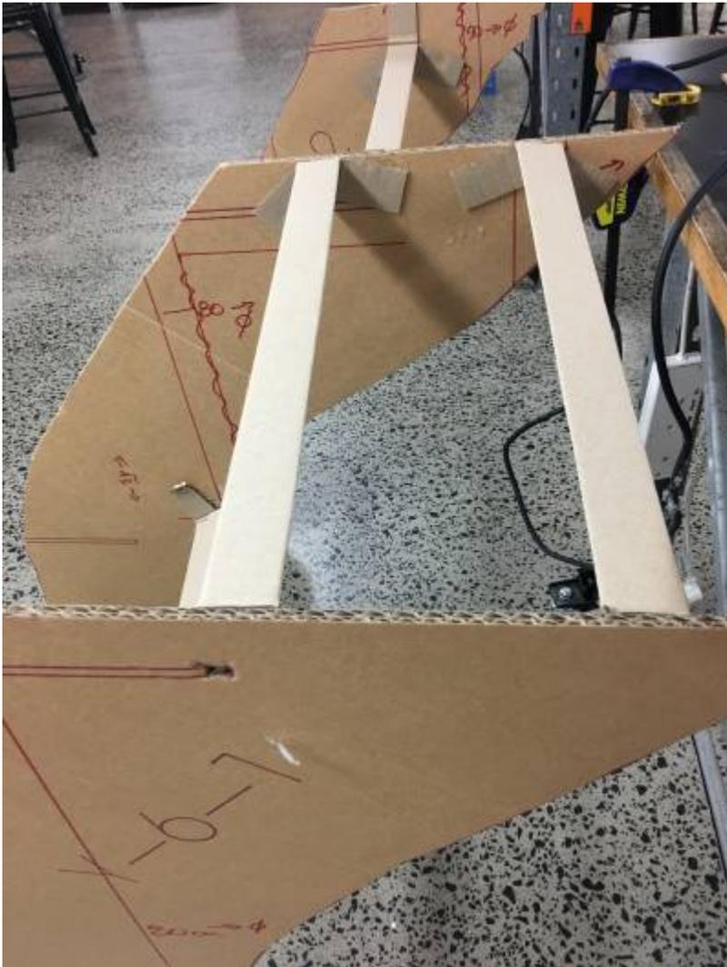
Ribs glued with a flat face flush to the top edge kept this face horizontal, and gave a surface for gluing on a top plate. (Note that one of the rib glue tabs has been removed, rather than bending it over the edge, and so introducing bumps).
