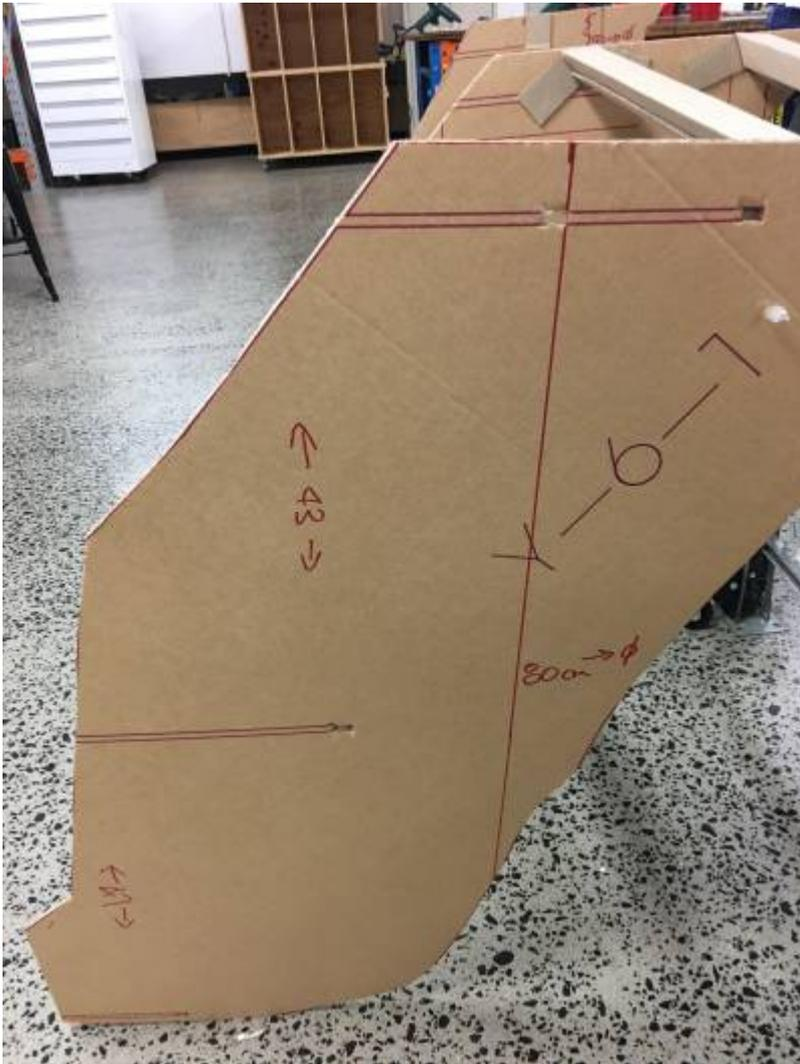
Suggestion: a system of registration lines is essential for future models. Adding a scaling key would also help to check that re-sizing had not been introduced.
