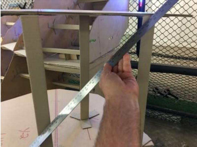
A rough measurement was made while the sections were held in place, and a single strip brace was made to help support the hanging piece.
