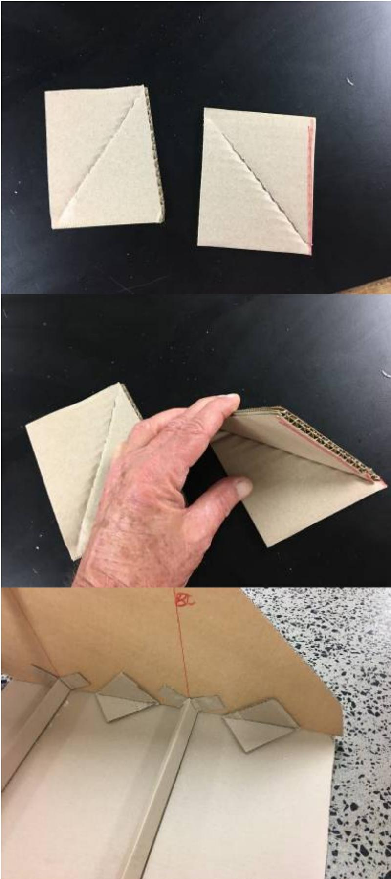
A few rough quadrilaterals were made from waste, then scored and folded along a diagonal axis.
