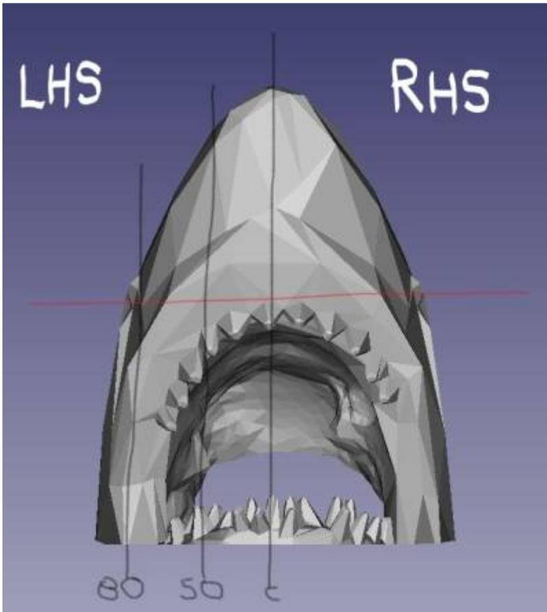
A vertical centre line was drawn on each Y-element, and then vertical registration lines drawn on each Y-element at 50 and 80 cm out from the centre. The Z-element slots that were in the design gave a horizontal to work from, and their irregular spacing allowed the heights to be kept aligned.
