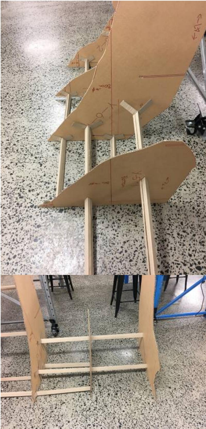
The support beams were pushed through the holes, and butted up to the adjacent Y-element. They were also located through holes in the next Y-element along to get them horizontal before gluing in place.
