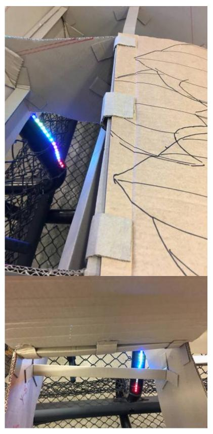
A few 50mm wide strips were cut to make the hinge, and thoroughly worked (crushed and bent over the edge of a bench) to make them almost circular. These pieces need to be long enough to reach loosley around the rib, with about 50mm at either end for gluing to the skin.
