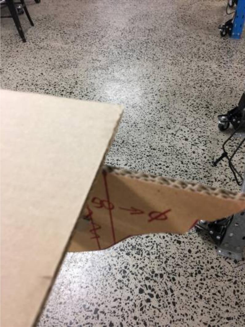
Use the registration marks to keep the Y-elements in place as you glue the plate down. Start with one section, and glue successive ones in place as you go, adjusting alignment as required.
