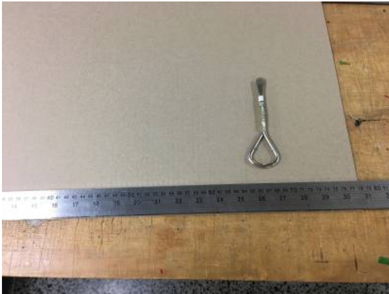
Rib layout, with scoring tool (use the ROUNDED corners so the cardboard is not cut)
