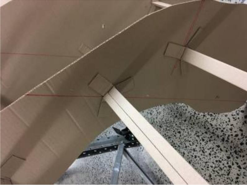
Aligning ribs to keep them horizontal and parallel to the centre axis of the model was an issue (another reason for lots of registration marks).
