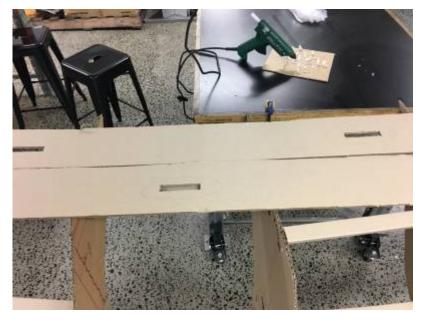
Mark and cut slots for the connectors. Note that these slots are THE WRONG WAY ROUND as the ribs beneath will interfere with the wedges. Slots should run perpendicular to the ribs.
