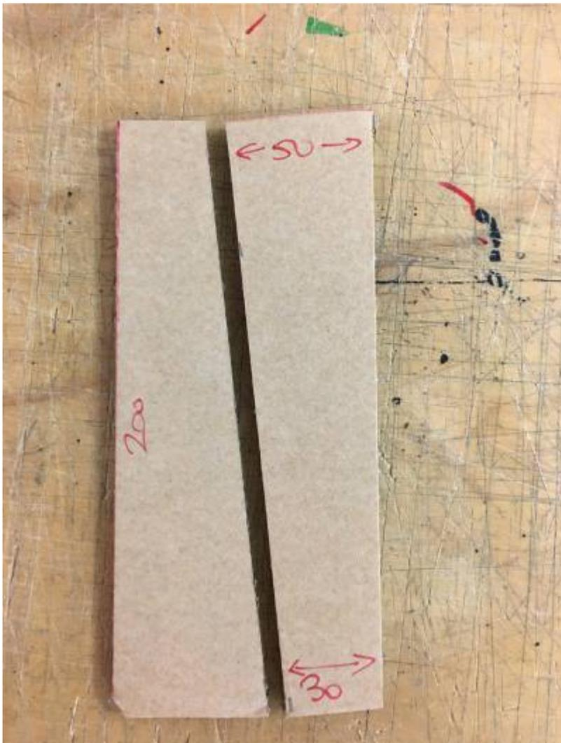
Cut out a couple of wedges, also made from 3 layers of 6mm cardboard.
