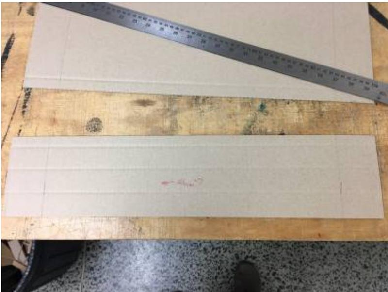
Cut the rib down the middle of the fourth parallel - this gives a gluing tab to both adjacent ribs.
