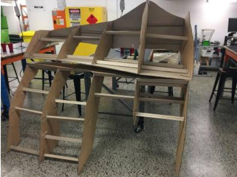
The registration marks were used to align the ends of the two module, but warping meant a good horizontal alignment was not achieved.
