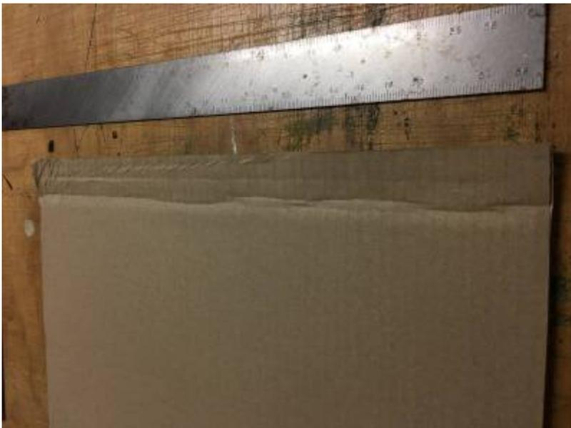
After measuring, a flap was cut, and worked to make a curved surface following the lines of the Y-elements. This means the flap might not always be a square piece. The edge where the flap is attached to the skeleton was crushed from both sides, to make a more flexible joint.
