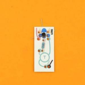
When you look at the back of the circuit board, two wires are now adjacent: the middle one from the transistor and one from the resistor.
