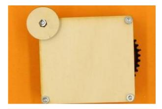
You may need to press down firmly on the bottom plate to attach nuts to the corner screws (pressure also helps keep the motor support in place).
