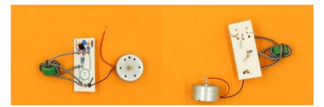
Now take the red wire on the motor, and push it through the hole at the end of the **red** line on the circuit.
