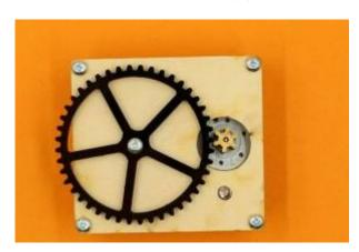
In the packet of wooden bits, there should be 12 small tubular spacers (you might have to pop them out of their carrier first). Put **three spacers** onto each screw (even though only two per leg are shown).
