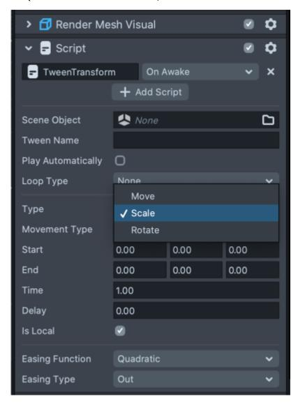
In the End fields add the scale of your model that you can see in the Transform section, for this example it is 0.40. The Start should be 0, as we want it to look like our leaf or mushroom is growing out of our head. We also want to set our main scale in the Transform window to 0, so the lens doesn't start with your object showing.
