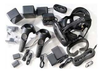
**3.** Install the 2 base stations on their stands, at opposite corners of your playing area, ensuring they have an unobstructed view of each other and no more than 5 metres apart. Connect their power supplies (with the right angle DC plugs) and power the units on. After booting they should display a green light and channel indicators. One station should display Channel B, one should display Channel C.
