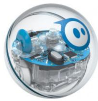
Sphero is a spherical robot that can be used with a range of apps (more than 30 available) on devices including tablets and smartphones. The robot shell is water proof and is made of tough, transparent polycarbonate, allowing students to see the relationship between their commands and the electric motor and LEDs inside.
