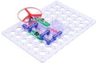
Components connect together using a plastic backboard and requires no previous electronics experience or soldering.
