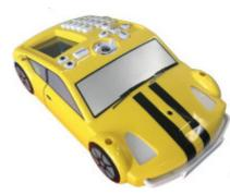
Pro-Bot is the grown up version of the Bee-Bot and can be programmed using robotic controls on the car or through Logo programming. This race car designed bot allows students to enter commands via a set of arrow and number keys mounted on the back. Plan a route for the Pro-Bot and press the corresponding keypad controls then press GO. The Pro-Bot also allows repeat loops and has bumper and light sensors to take programming to the next level.
