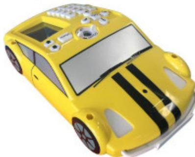
Pro-Bot is the grown up version of the [Bee-Bot](#) and can be programmed using robotic controls on the car or through Logo programming. This race car designed bot allows students to enter commands via a set of arrow and number keys mounted on the back. Plan a route for the Pro-Bot and press the corresponding keypad controls then press GO. The Pro-Bot also allows repeat loops and has bumper and light sensors to take programming to the next level.
